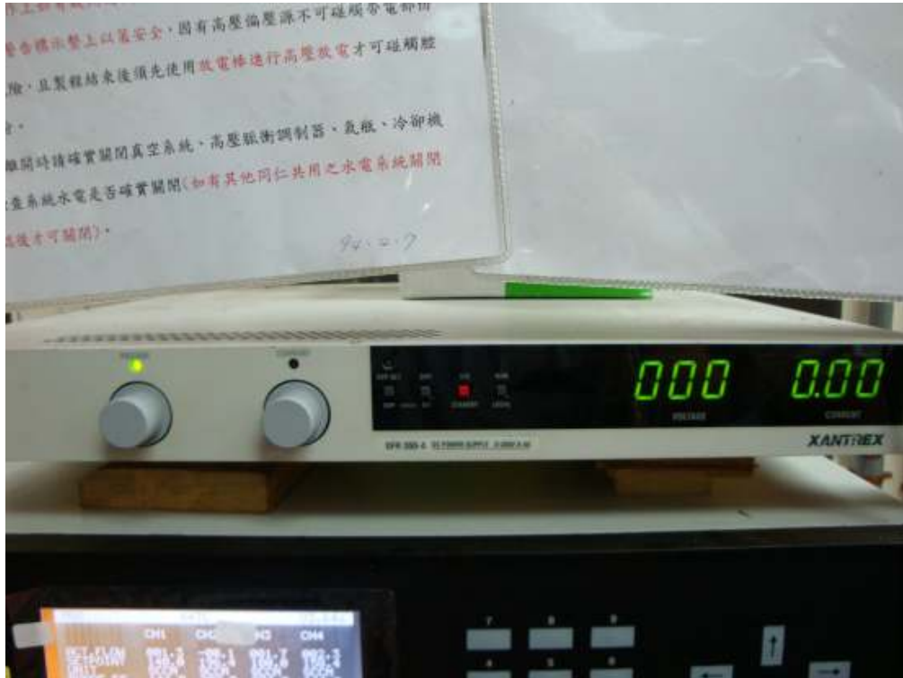
Fig.1-4. The DC power supply of electrical power system
