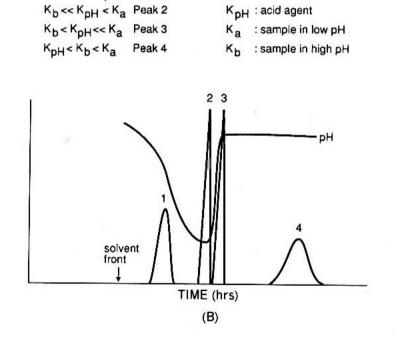
圖一 酸鹼區域精鍊法示意圖(取自 p128,"High-speed Countercurrent Chromatography"Edited by Y. Ito and W.D. Conway, John Wiley \$ sons, Inc. 1996)
