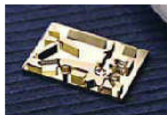
Microoptical assembly board for a distance sensor.
