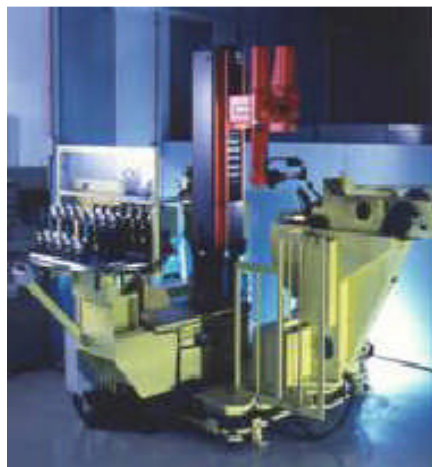
圖 5-11 Automated aerofoil restoration
