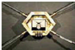
Microoptical fiber switch with electrostatic actuator.
