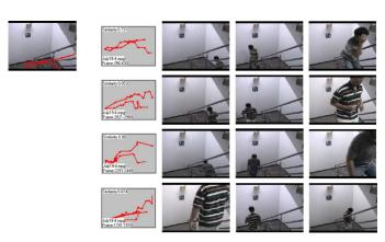
Fig. 12. Example of the retrieval result using query-by-sketch in a stairway scenario. The top four retrieved results (out of 108 video clips) are all related video clips.
