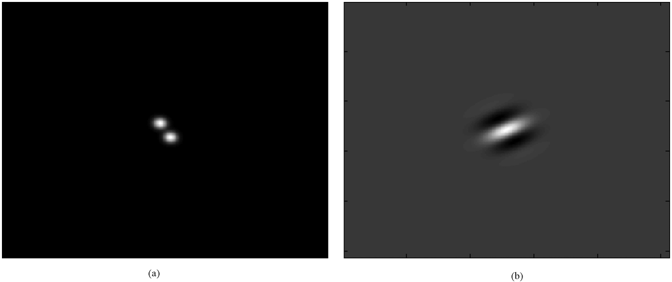
Fig. 3. Example of 2-D Gabor type filtering. (a) Standard 2-D Gabor type filter in time domain. (b) In frequency domain.
