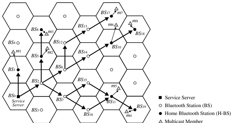
Fig. 2. A constructed multicast tree obtained by executing the existing unicast protocol repeatedly.
