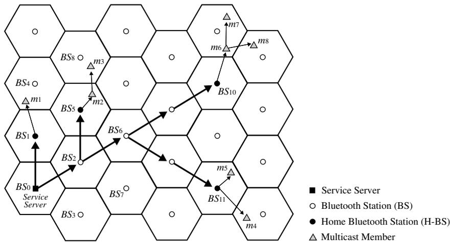
Fig. 3. A constructed multicast tree obtained by applying the proposed multicasting protocol.
