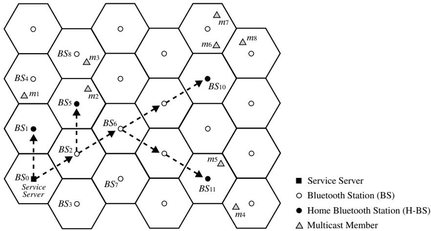
Fig. 5. The multicast tree constructed by applying the MRC phase of RCMP.
