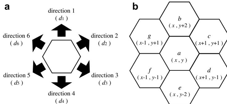
Fig. 4. The possible directions and relative coordinates of each cell: (a) six possible directions for packet forwarding, (b) relative coordinates in BLN.
