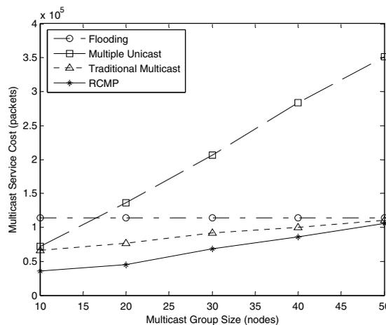
Fig. 12. Comparison of multicast service costs with variant in multicast group size.
