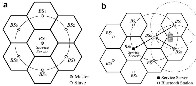
Fig. 1. Bluetooth Location Network architecture: (a) Bluetooth Stations and Service Server in a BLN, (b) example of obtaining location information of a Bluetooth mobile device in BLNs.
