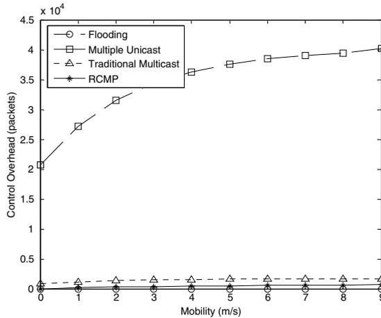
Fig. 9. Comparison of control overheads when considering mobility.
