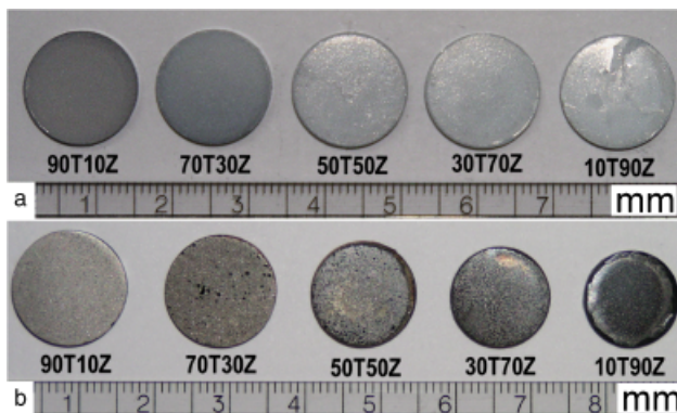
Fig. 1. (a) Ti/ZrO 2 green bodies; (b) sintered composites after sintering at 1500°C/1 h in argon.
