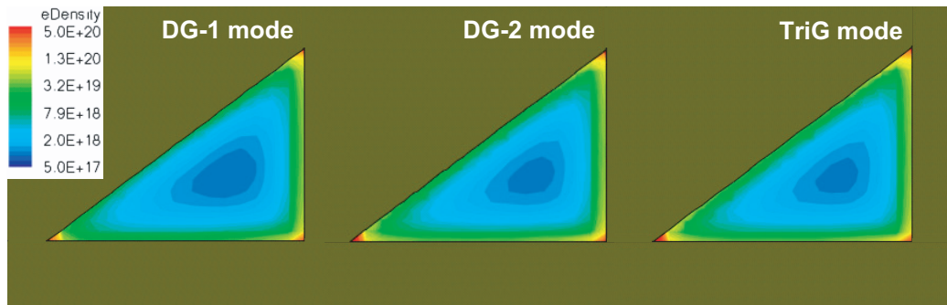
Figure 5. Two-dimensional simulation of electron density (eDensity) in NWs under DG-1, DG-2 and TriG modes of operation. The applied gate voltage is 5 V.
