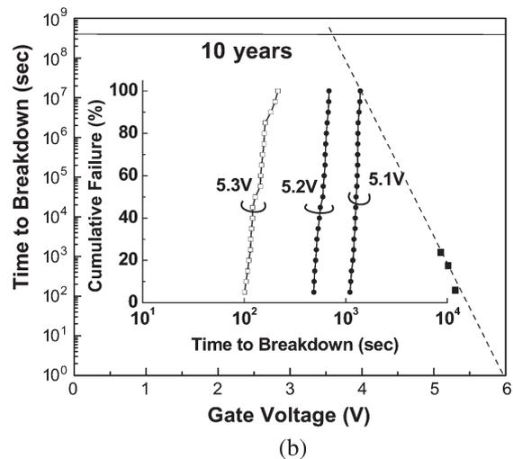
Fig. 4. (a) Electron mobility extracted from the  $I_d - V_d$  characteristics of an  $\text{YbSi}_{2-x}/\text{HfAlON}$  n-MOSFET and (b) the time-to-breakdown distribution and maximum operation voltage plots.
