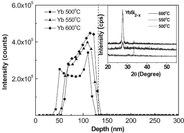
Fig. 2. SIMS of Yb in the  $\text{YbSi}_{2-x}/\text{HfAlON}$  structure. The inset figure is the XRD profiles.
