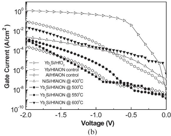
Fig. 1. (a)  $C-V$  and (b)  $J_g - V_g$  characteristics for  $\text{YbSi}_{2-x}/\text{HfAlON}$ ,  $\text{Yb}/\text{HfAlON}$ ,  $\text{Ni}/\text{HfAlON}$ , and  $\text{Al}/\text{HfAlON}$  capacitors, measured under accumulation. The device area was  $100 \mu\text{m} \times 100 \mu\text{m}$ .
