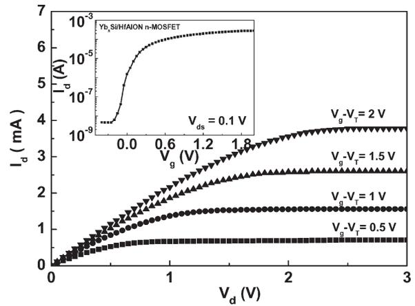
Fig. 3.  $I_d - V_d$  characteristics of an  $\text{YbSi}_{2-x}/\text{HfAlON}$  n-MOSFET. The inset figure is  $I_d - V_g$  curves. The gate length was  $10 \mu\text{m}$ .
