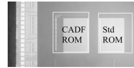
Fig. 7. Die photos of a 256-Kb conventional (Std) ROM with X pattern and a 256-Kb CADF ROM ( k = 8 , n = 16 , and m = 32 ) with X pattern.
