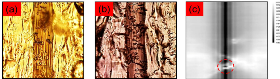
Fig. 4. Microscope images of sliced (a) durable and (b) poorly-durable polarizers. (c) The two-photon absorption virtual biopsy image of the test polarizer. Image sizes in these three figures are 100 \mu\text{m} by 100 \mu\text{m} . The PVA layers are vertically located in the center of the three figures with a 25 \mu\text{m} thickness.
