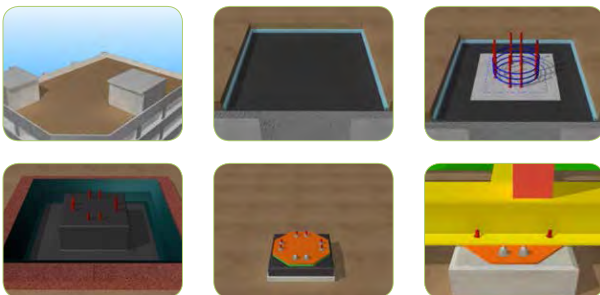
Structural connection between the Orchid House and existing building
