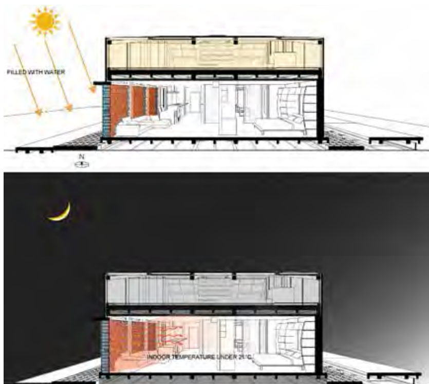
Thermal wall experiment diagram
