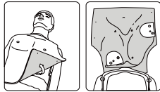
Installing the Internal Manikin Adapter MS088A with the Loréal Resuscitator.
