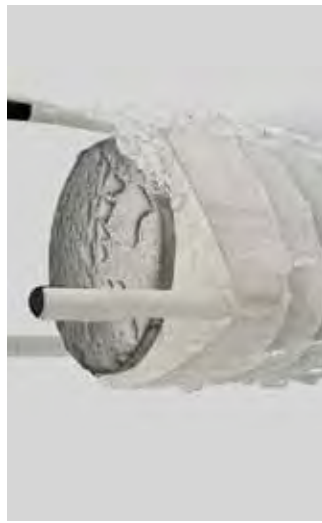
The WXT520 has an automatic control circuit that switches the heating on at low temperatures.
