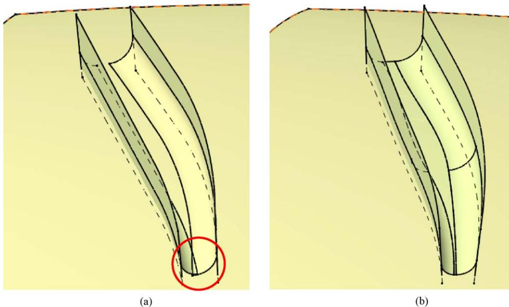
Fig. 18. (a) Intersection of rounding surfaces and (b) automatic correction of the intersection.
