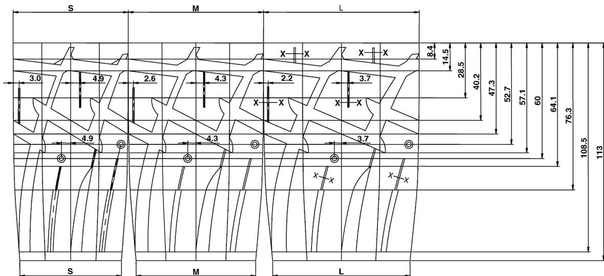
Fig. 2. Three pitches (small, medium, and large) in a tire design.
