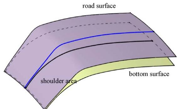
Fig. 10. Shoulder area in a tire mold.
