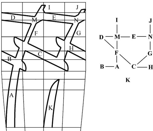
Fig. 4. Connectivity of a groove pattern in one pitch and its non-directional graph.
