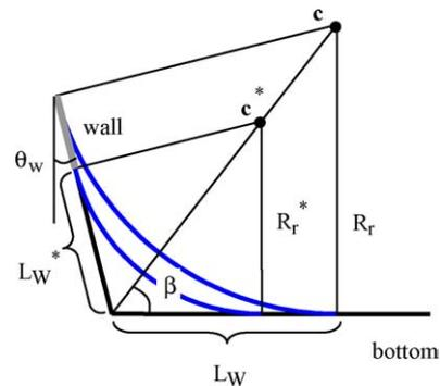
Fig. 14. Adjustment of rounding radius in a shallow groove.
