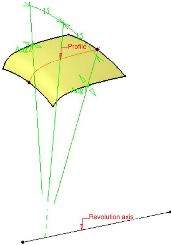
Fig. 5. Construction of the road/bottom surface by revolving a profile along a given axis.
