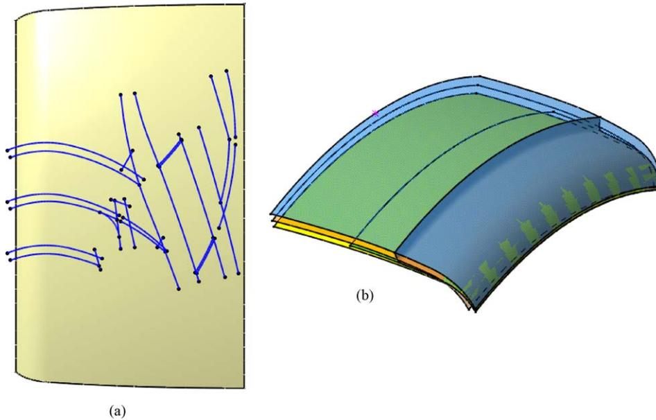
Fig. 15. (a) Guide curves of one pitch extracted with tire design importer and (b) road and bottom surfaces.
