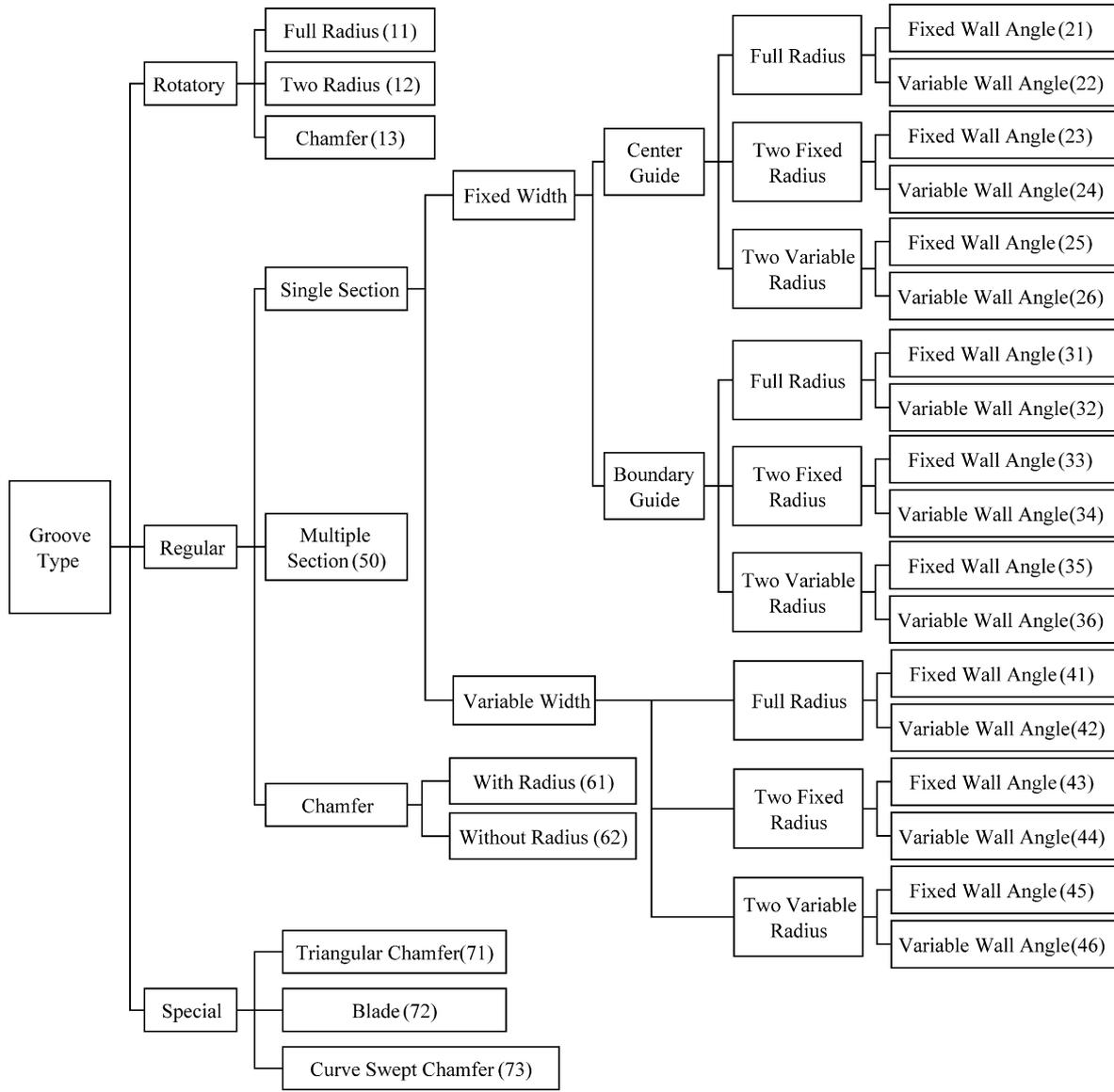
Fig. A.1. Classification of common groove shapes.
