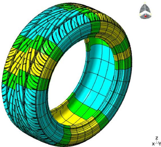
Fig. 22. Complete 3D tire mold constructed with the proposed system.
