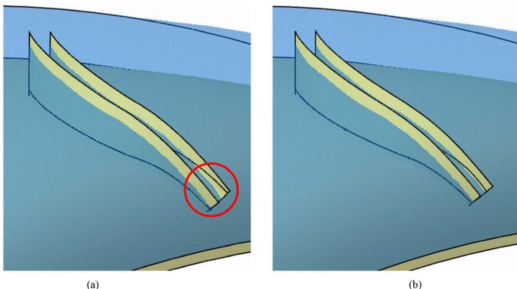
Fig. 20. (a) The rounding surface protrudes out of the road surface near the shoulder area and (b) automatic correction of the rounding surface protrusion.
