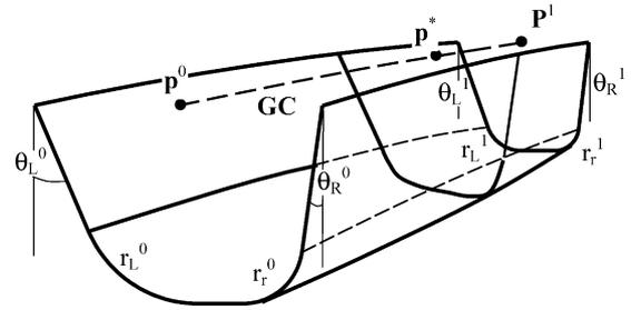
Fig. 7. Construction of groove shape by lofting cross-sectional profiles.
