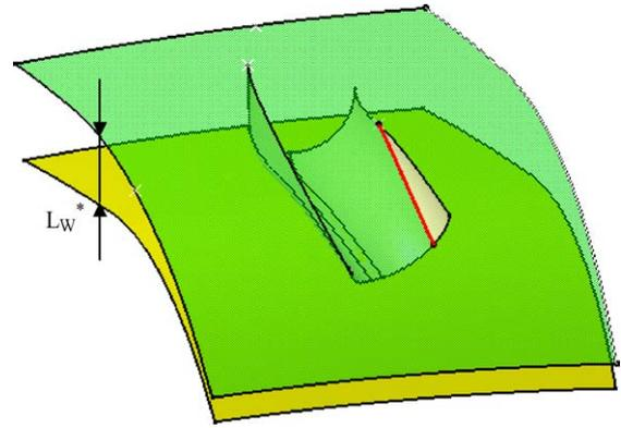
Fig. 13. Blending operation fails at shallow grooves.
