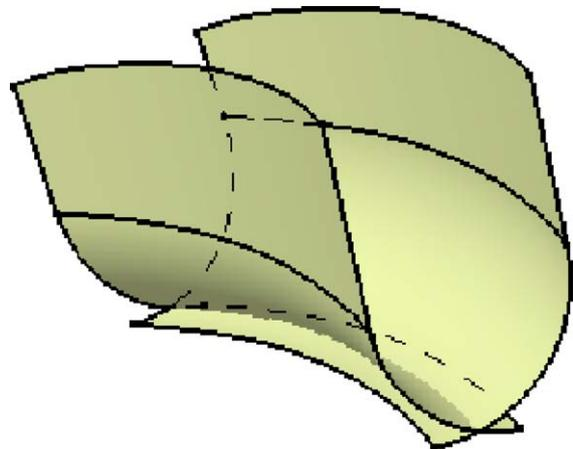
Fig. 8. Intersection of rounding surfaces.
