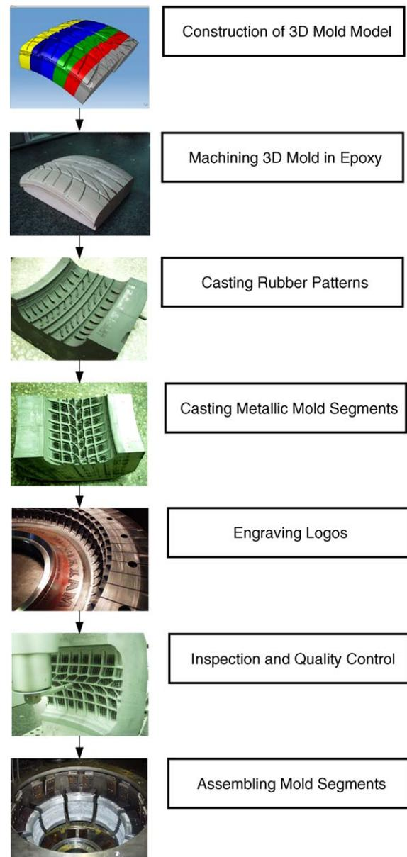
Fig. 1. Production procedure of a segmented tire mold.
