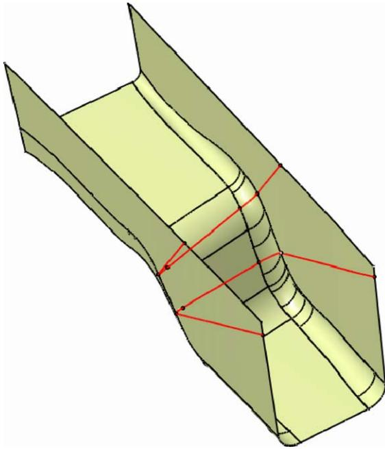
Fig. 19. Elimination of the surface crease caused by the intersection of lofting profiles.
