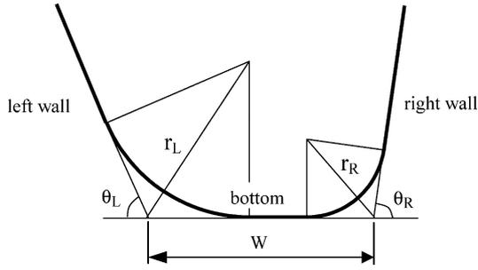
Fig. 9. Definition of the width in a groove cross-section.
