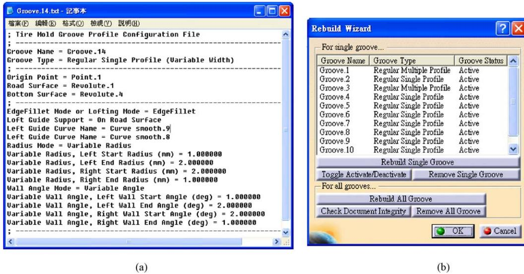
Fig. 17. (a) Groove parameter values in a text file and (b) GUI in parametric design coordinator.
