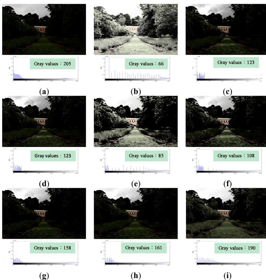
Figure 6. Comparison results for the image “Landscape” [23] (image size: 596 \times 397 pixels). (a) Original image; (b) Histogram Equalization (HE); (c) Bi-histogram equalization (BBHE); (d) Recursive mean-separate histogram equalization (RMSHE) ( r = 2 ); (e) Dualistic sub-image histogram equalization (DSIHE); (f) Recursive sub-image histogram equalization (RSIHE) ( r = 2 ); (g) Bi-histogram equalization with a plateau level (BHEPL); (h) Dynamic quadrants histogram equalization plateau limit (DQHEPL); (i) Visual contrast enhancement algorithm (VCEA).
