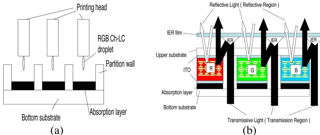
Fig. 7. Full-color transfective Ch-LCD can be obtained by (a) first patterning RGB Ch-LC with IJP on bottom substrate with an absorption layer and partition wall and then (b) laminating IER film on the upper substrate and well aligning to the bottom substrate. (Color version available online at <http://ieeexplore.ieee.org>.)
