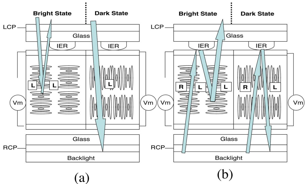
Fig. 1. Schematics of the proposed transfective Ch-LCD for (a) reflective mode and (b) transmissive mode. (Color version available online at <http://ieeexplore.ieee.org>.)
