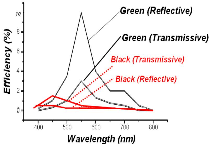
Fig. 4. Measured spectrum of the transfective Ch-LCD with IER film by ConoScope. (Color version available online at <http://ieeexplore.ieee.org>.)
