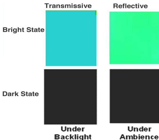
Fig. 5. Photographs of monochromatic transfective Ch-LCD with IER film in transmissive mode under backlighting in a dark room and in reflective mode under office lighting. (Color version available online at <http://ieeexplore.ieee.org>.)
