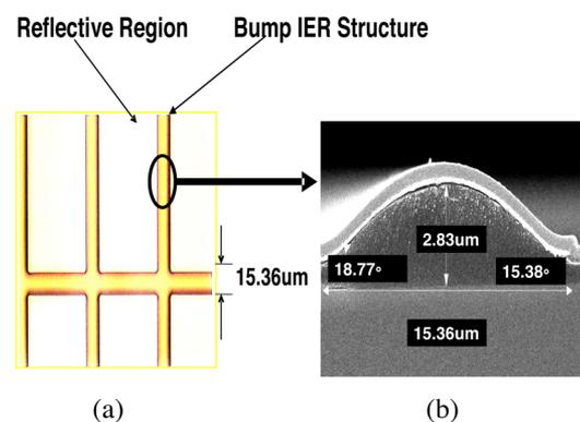
Fig. 3. (a) Fabricated IER film measured by Optical Microscope and (b) cross section of the bump-IER structure by SEM at reflowing temperature of 14°C. (Color version available online at <http://ieeexplore.ieee.org>.)
