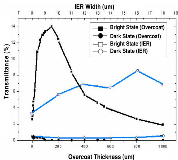
Fig. 2. Transmissive light efficiency in bright and dark states with various OC thicknesses and IER width. (Color version available online at <http://ieeexplore.ieee.org>.)
