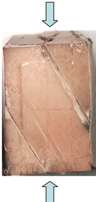
Fig. 7. Shear failure mechanism for 30° specimen.
