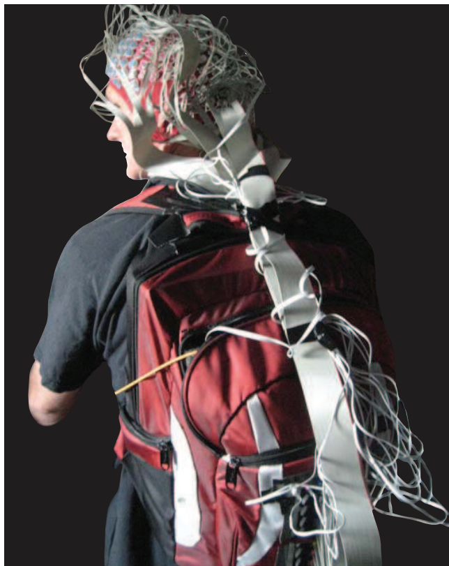
FIGURE 2. State-of-the Art Laboratory Grade EEG System made “Mobile.” Participant wears a high-density wet-electrode cap which is wired to a laptop and amplifiers in a backpack. This system takes approximately 1 hour to set-up, and can become uncomfortable in minutes.
