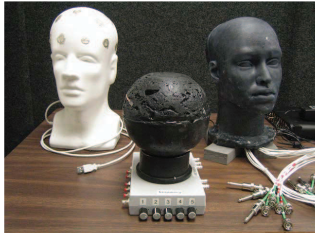
FIGURE 7. Sample prototype “phantom head” devices developed under the SBIR program. Models provided by CFDRC (left), POC (center), and Creare (right) are designed to be conductively analogous to the human head, with embedded sources to create realistic electrical dipoles detectable at the surface.
