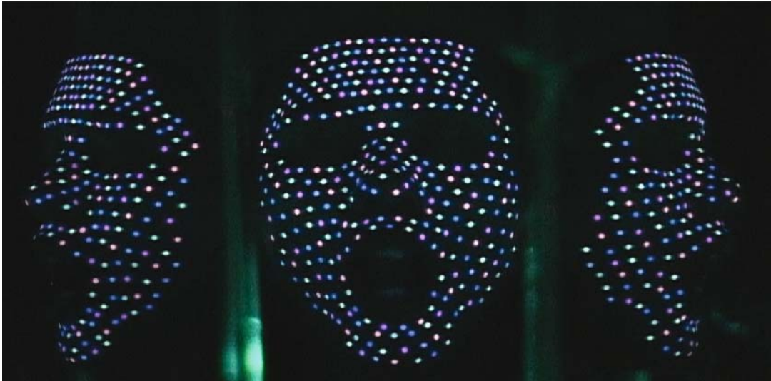
Fig. 3. A captured video clip of fluorescent markers illuminated only by BLB lamps. The fluorescence is visible in the visible light spectrum and no special lens is required for filtering
