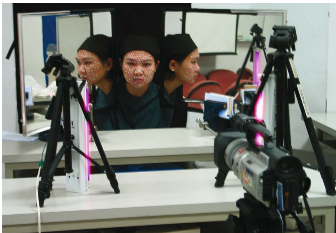
Fig. 2. The tracking equipment. This photo is taken under normal light. Two “Blacklight Blue”(BLB) lamps are placed in front of a subject and mirrors. The low-cost special lamps are coated with fluorescent powders, and it can emit long wave UV-A radiation to excite luminescence
