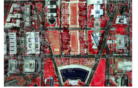
Fig. 12. False-color IR image of a portion of Washington, DC mall image measuring 205 \times 307 pixels. There are seven categories: Grass, tree, roof, water, road, trail, and shadow.
