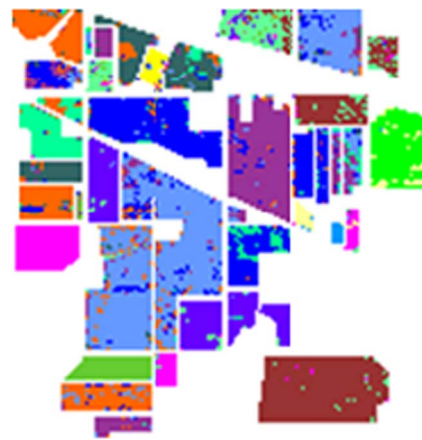
Fig. 2. SVM classification result of the IPS image, containing specklelike errors.
