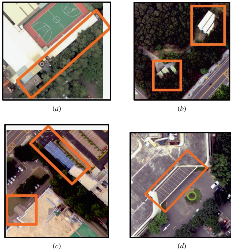
Figure 15. Omission error examples in building region generation. (a) Vegetation occluded. (b) Few light detection and ranging (LIDAR) points. (c) Ground detection error. (d) Lack of LIDAR points.
