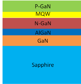
Fig. 1. Schematic diagram of the GaN-based LED without the pyramid texture.
