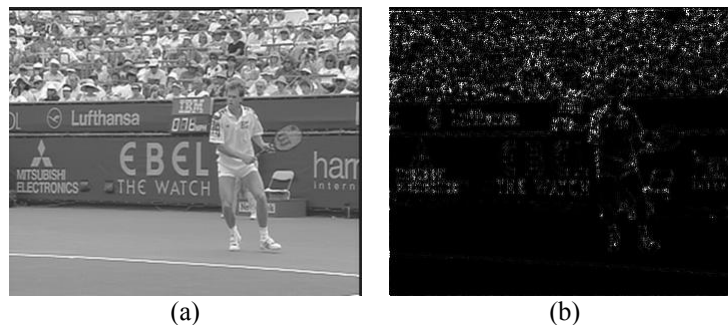
Figure 4: An image and its Hessian value. (a) The image. (b) The Hessian value.
