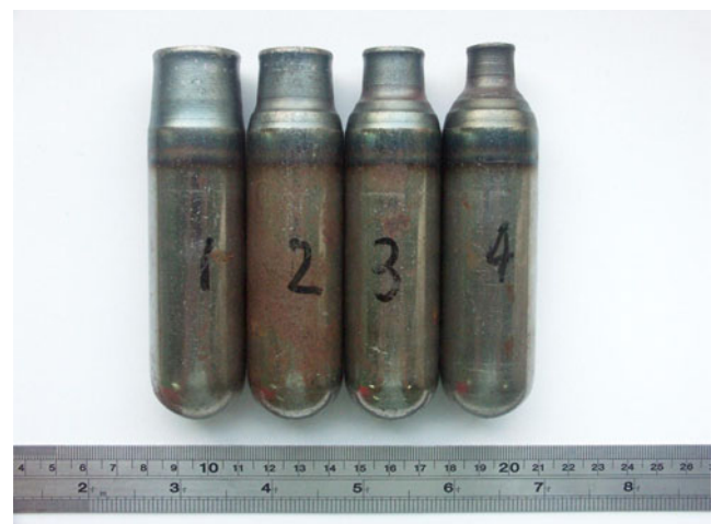
Fig. 5 Four stages of spun tubes
