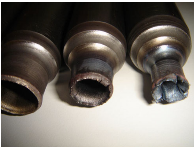
Fig. 1 Fracture after spinning at room temperature
