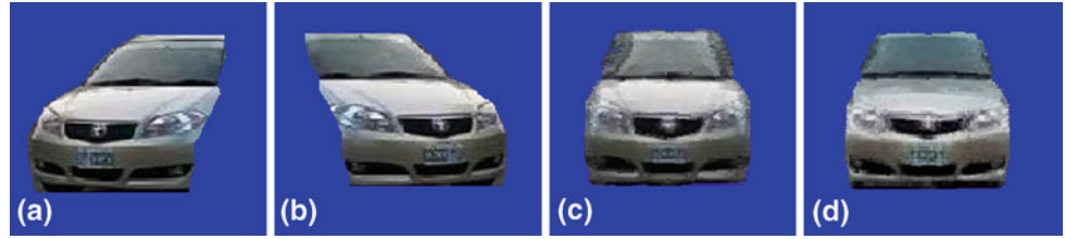
Fig. 6 a Segmented image of front region, b mirror image of a , c synthesized car image from a and b by mirror morphing, d synthesized template car image
