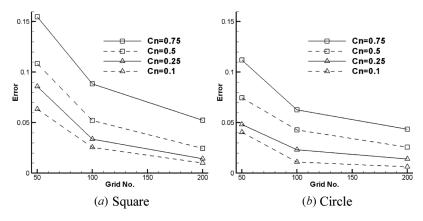
Figure 5. Numerical error against grid number for advection of cylinders in uniform flow.
