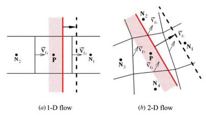
Figure 2. Advancing of interface through the face of a control volume (color figure available online).
