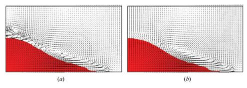
**Figure 8.** Flow field for the collapse of water column: (a) with one smoothing step; (b) with two smoothing steps (color figure available online).
