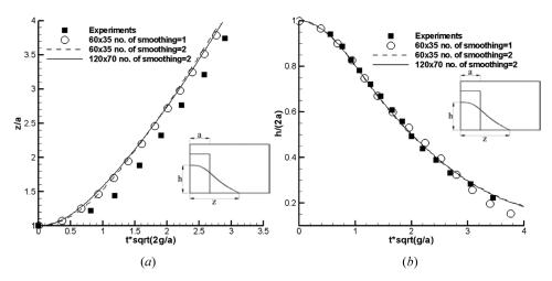
**Figure 9.** The collapse of water column: (a) position of the leading front edge along the floor; (b) height of the retreating front along the wall.
