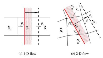
Figure 3. Retreating of interface through the face of a control volume (color figure available online).
