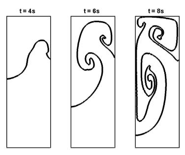
Figure 12. Evolution of Rayleigh-Taylor flow obtained using 96 \* 288 grid.
