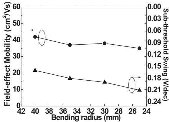
Fig. 5. Field-effect mobility and sub-threshold swing as a function of bending radius for IGZO/YTY TFT.
