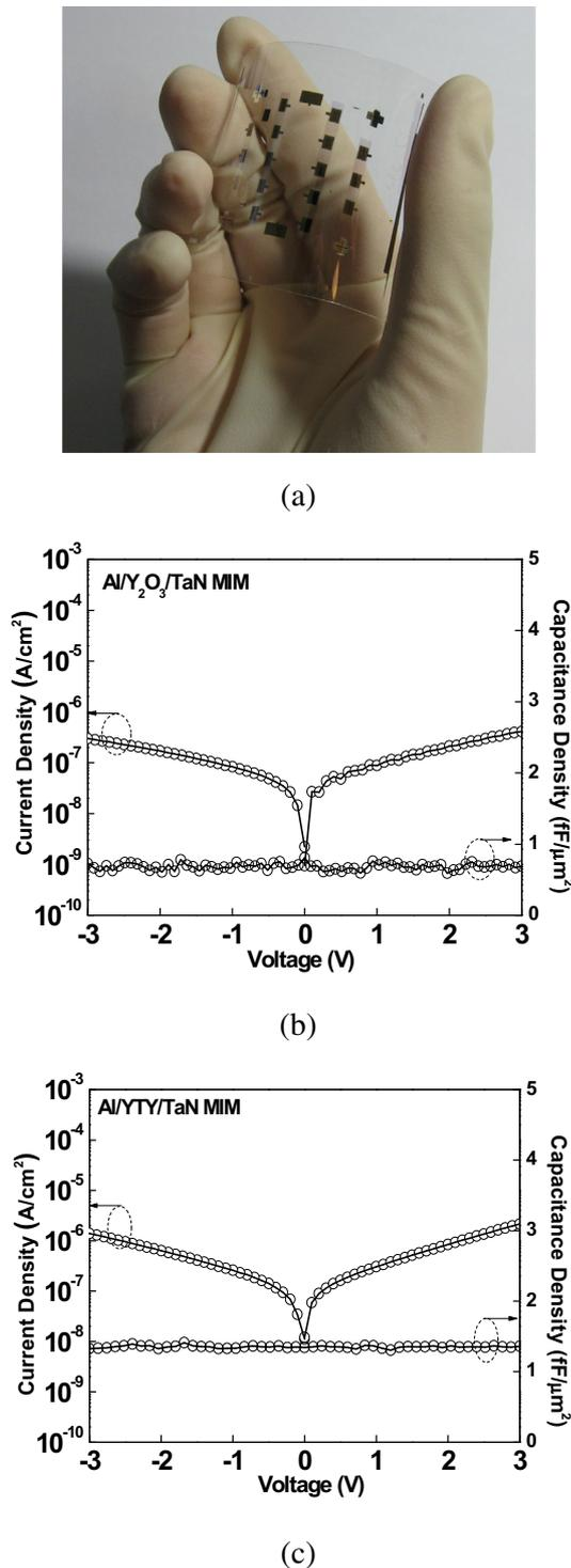
Fig. 1. (a) Photograph of flexible and transparent IGZO TFTs.  $C$ – $V$  and  $I$ – $V$  characteristics of (b) Al/Y<sub>2</sub>O<sub>3</sub>/TaN and (c) Al/YTY/TaN MIM capacitors on flexible PC substrates.
