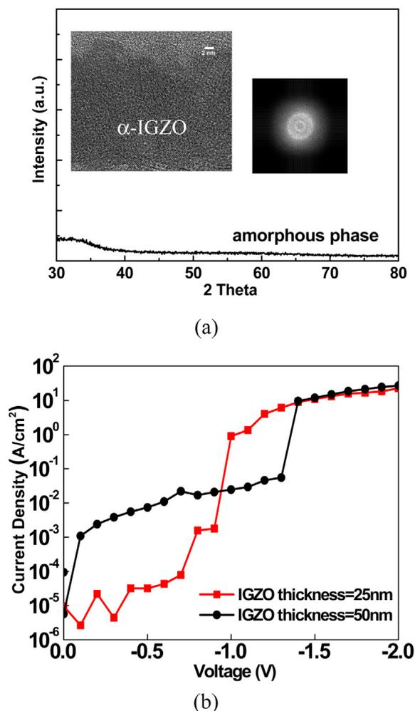
**Fig. 3.** (a) XRD spectrum of IGZO channel layer and (b)  $I$ – $V$  characteristics of Al/IGZO/TaN MIM capacitors with different IGZO thicknesses. The high-resolution TEM and FFT images of IGZO channel were inserted in Fig. 4(a).
