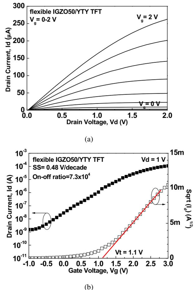
Fig. 2. (a)  $I_d$ – $V_d$  and (b)  $I_d$ – $V_g$  characteristics of flexible YTY TFT with 50-nm-thick IGZO channel layer.
