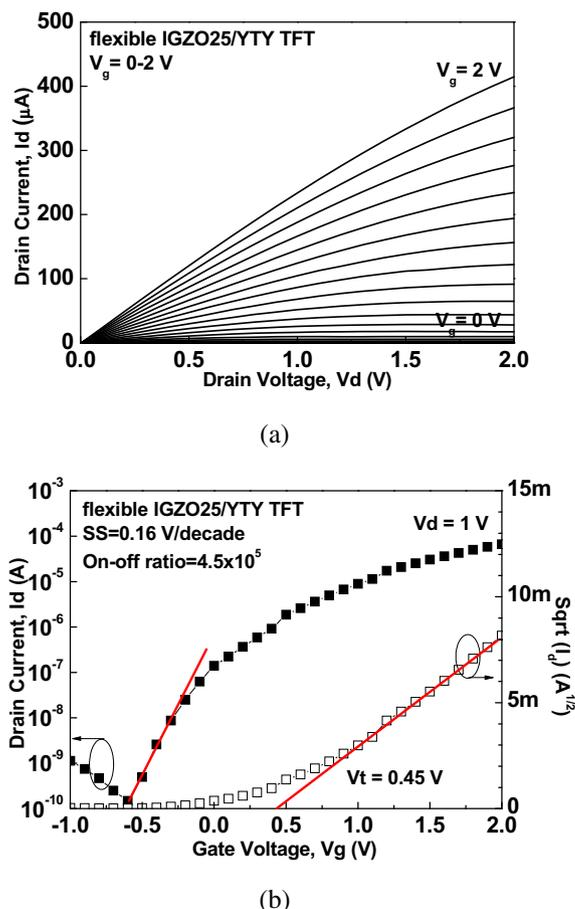
**Fig. 4.** (a)  $I_d$ – $V_d$  and (b)  $I_d$ – $V_g$  characteristics of flexible YTY TFT with 25-nm-thick IGZO channel layer.
