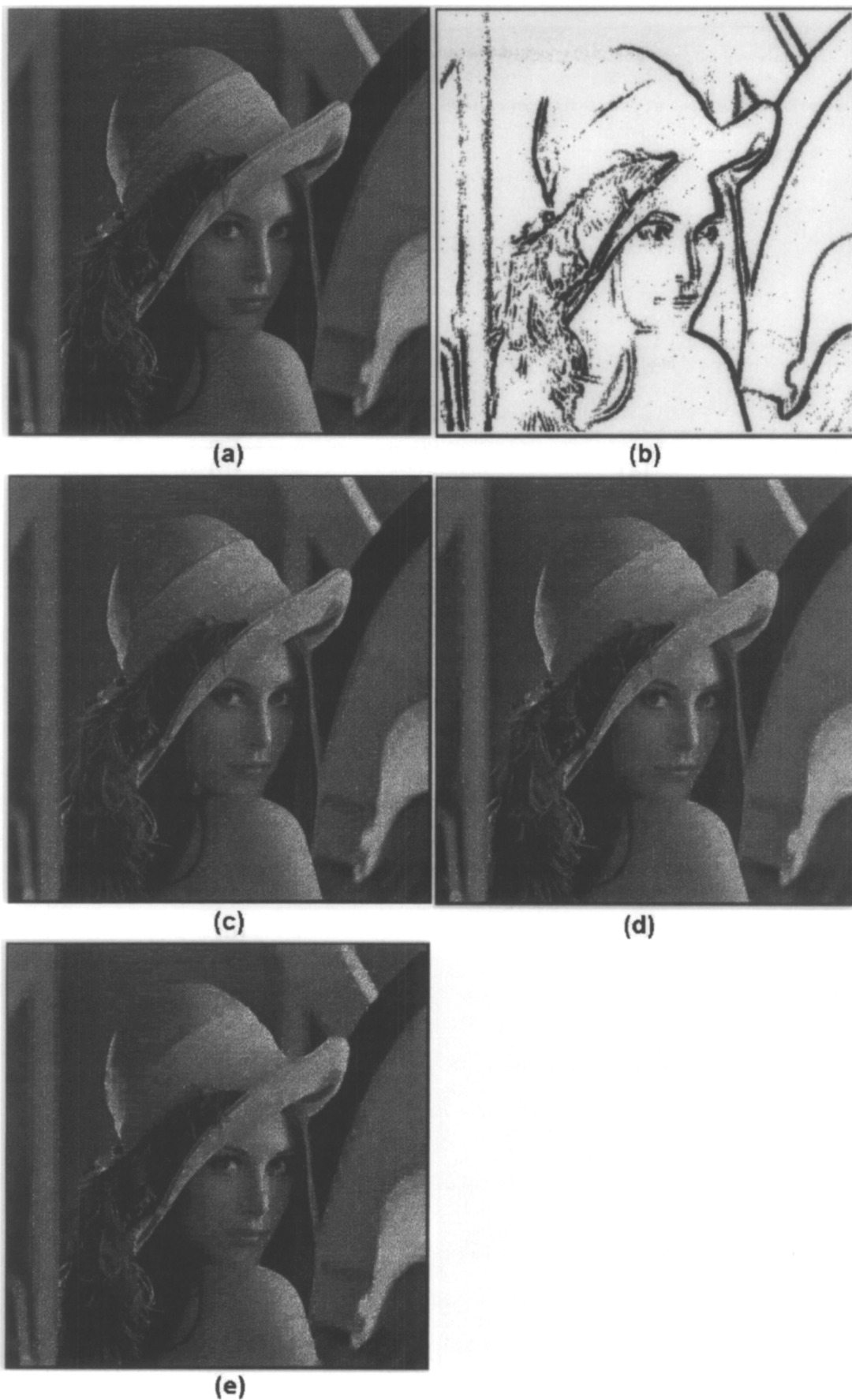
Fig. 4. The resulting images generated by using the proposed edge detection and compression methods to the image 'Lena'. (a) The original (input) error-diffused image, (b) the detected edge image for (a). The reconstructed images are: (c) CR=2, (d) CR=3, (e) CR=4. Note that (c)–(e) are all error-diffused (binary) images instead of gray-level (256-level) images.
