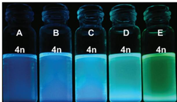
Fig. 5 Concentration-dependent emission phenomenon of compound **4n** at concentrations of  $5.0 \times 10^{-5}$  (A),  $7.5 \times 10^{-5}$  (B),  $1.0 \times 10^{-4}$  (C),  $2.0 \times 10^{-4}$  (D), and  $4.0 \times 10^{-4}$  (E), respectively.
