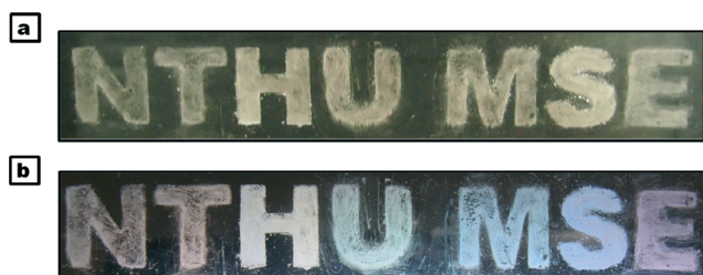
Fig. 5 Photographs of transparent plastic slides which were coated with the various-sized spheres by doctor-blade. (a) All the spheres synthesized with different concentrations of HMTA ( 40\text{--}140\text{ mM} ) have a white color which is similar to general ZnO powders. (b) When a back light is turned on, multicolored words could be observed through the transparent plastic slides by Mie scattering at a scattering angle of \theta > 0^\circ (from left to right, red (S4), orange (S6), yellow (S8), green (S10), cyan (S12), blue (S13), and purple (S14), respectively).
