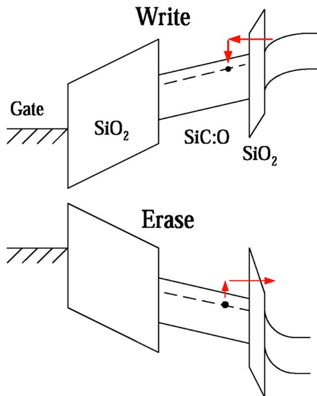
**Figure 3.** The band diagrams of the “write” and “erase” operation.
