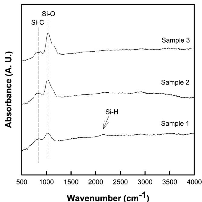
**Figure 4.** FTIR spectrum of the deposited SiC:O film.
