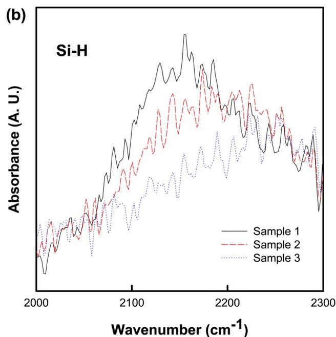
**Figure 5.** (a) The FTIR absorbance of Si-C bonds and (b) FTIR absorbance of Si-H bonds.
