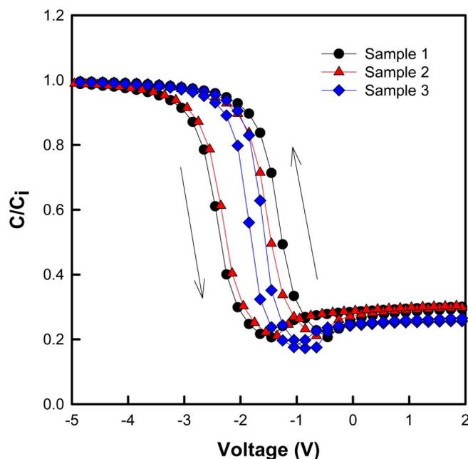
**Figure 2.** The C-V hysteresis for different samples under 7 and (-7) V bidirectional voltage sweeping.
