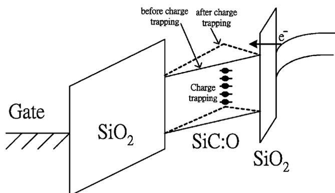
**Figure 8.** The band diagram shows that when the electrons are captured in a charge-trapping layer with rich charge-trapping sites, the conduction band of the charge-trapping layer is lifted, which forms an energy barrier for conductive electrons.
