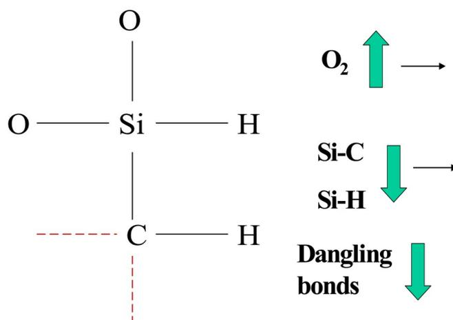
**Figure 6.** The structural formula of the proposed model. As the oxygen content is increased, both Si-C and Si-H bonds may be decreased, which renders the decrease of the dangling bonds. The dotted lines indicate the dangling bonds of the C-H bonds which are not well-bound.
