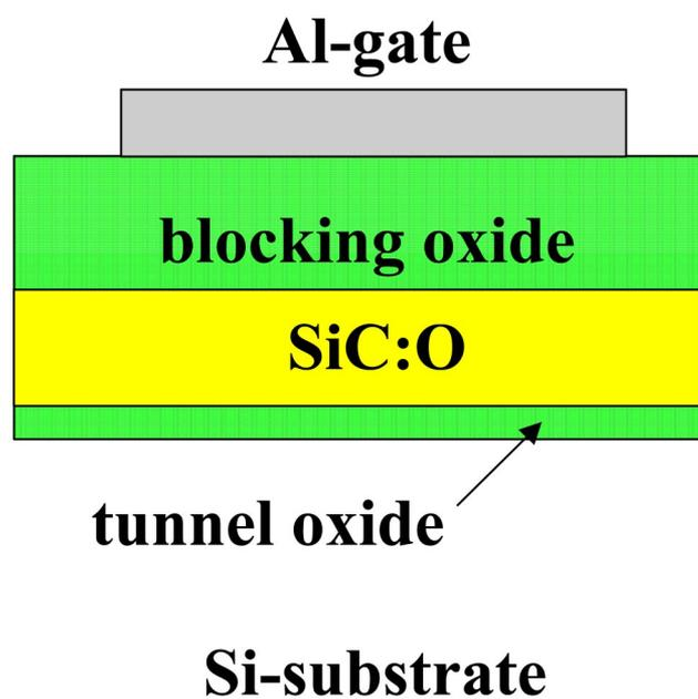
Figure 1. The structure of the MOIOS device shown in this work.
