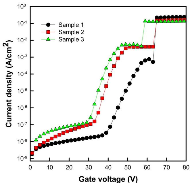
**Figure 7.** The leakage current characteristics of the sandwiched structure. The breakdown voltage is increased with the decrease of oxygen content.
