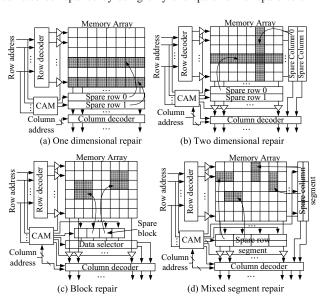
Fig. 1. Redundancy structures for memory repair.
