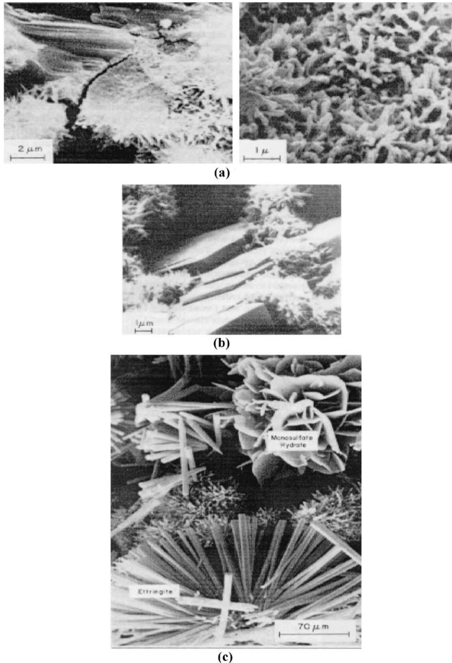
Fig. 10. Typical SEM Microstructures of (a) C–S–H, (b) CH and (c) Ettringite(Aft) and Monosulfate(Afm).
