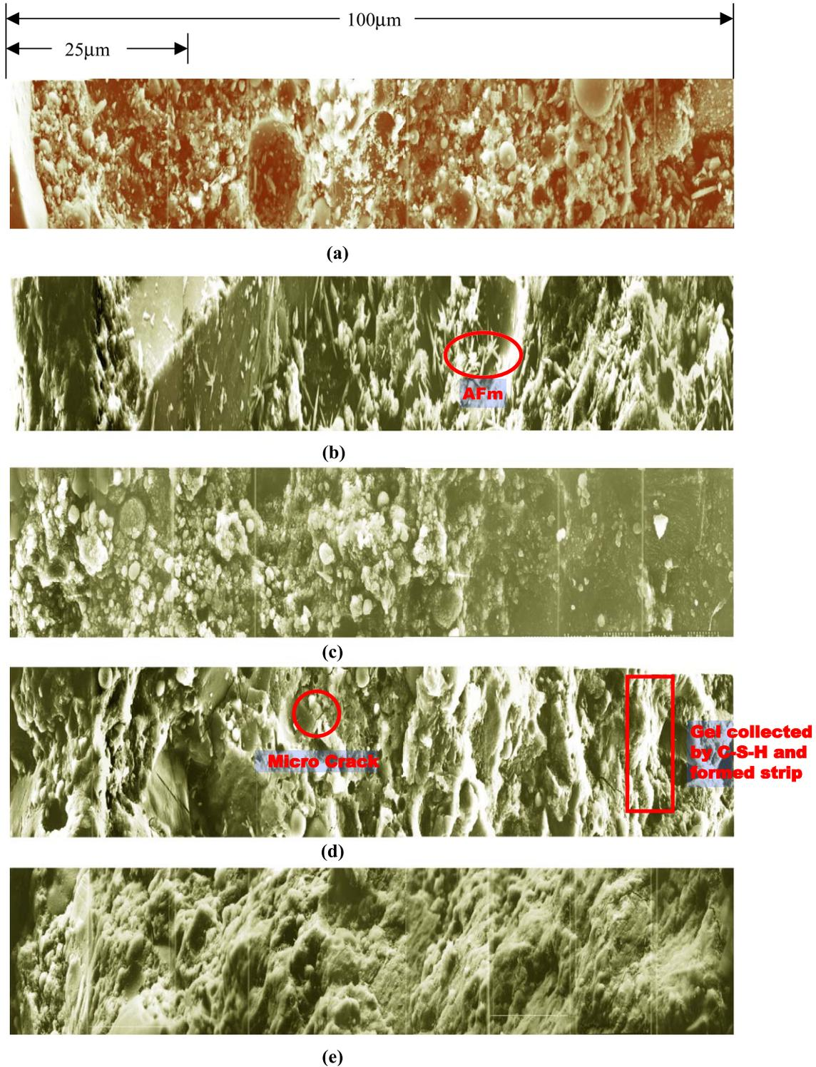
Fig. 9. Typical SEM Microstructures of transition zone of concrete curing with saturated lime water. (a) Typical SEM microstructures of the transition zone for 1 day (W/B=0.35); (b) Typical SEM microstructures of the transition zone for 7 days (W/B=0.45); (c) Typical SEM microstructures of the transition zone for 14 days (W/B=0.54); (d) Typical SEM microstructures of the transition zone for 28 days (W/B=0.54); (e) Typical SEM microstructures of the transition zone for 56 days (W/B=0.54).
