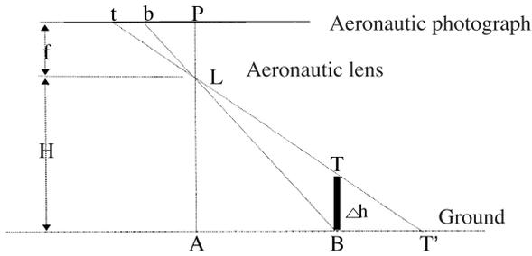
Fig. 6. Parallax variation of an aeronautical photograph.
