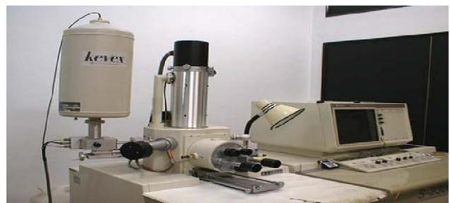
Fig. 5. Scanning electron microscope.
