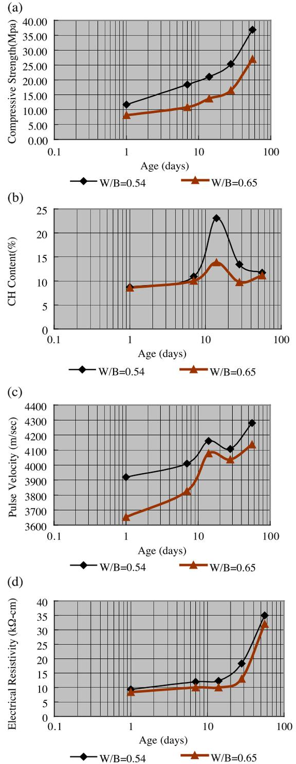
Fig. 18. The transmutation of (a) compressive strength, (b) CH content, (c) pulse velocity and (d) electrical resistance with different curing ages.
