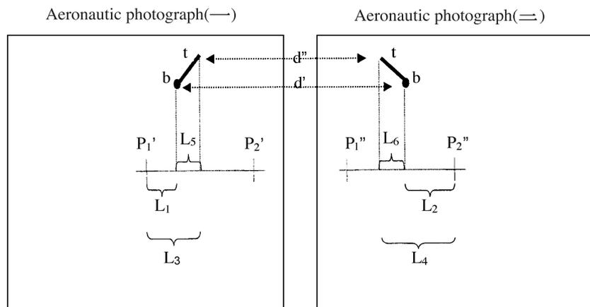
Fig. 7. The relationship of parallax by body TB at difference photograph.
