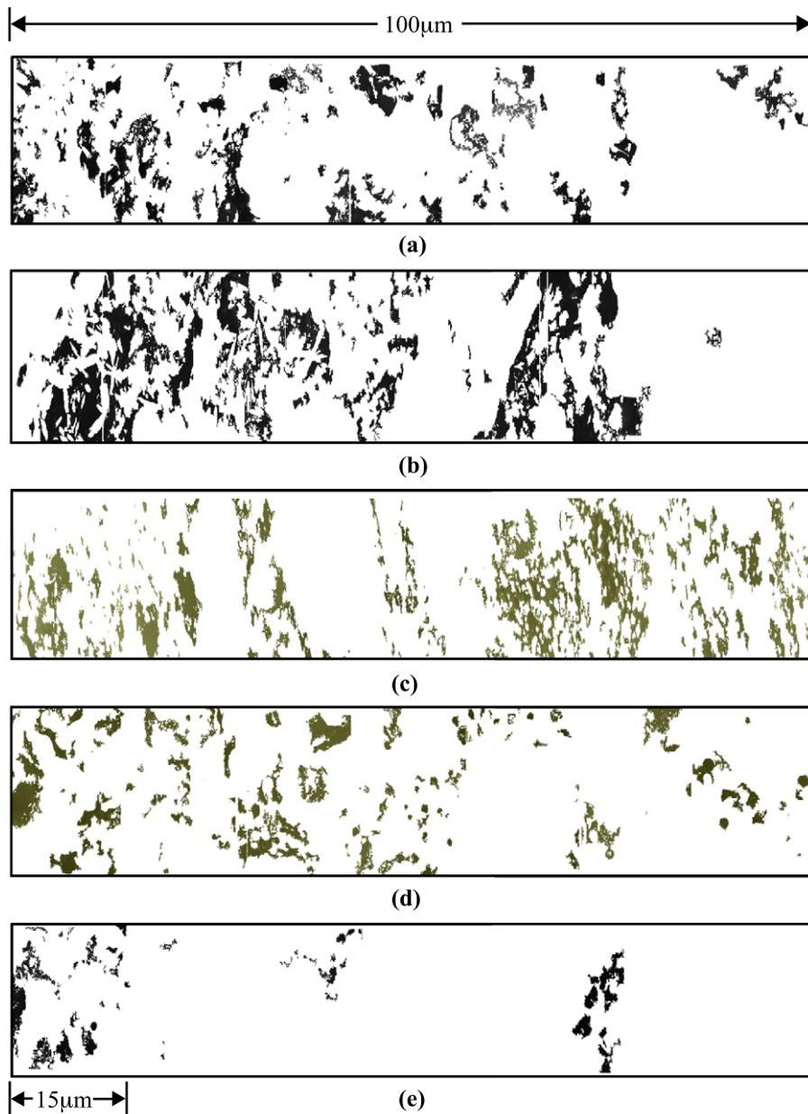
Fig. 12. The pore distribution of transition zone of concrete curing with saturated lime water (W/B=0.65) at (a) 1 day (porosity=20.44%), (b) 7 days (porosity=19.01%), (c) 14 days (porosity=16.56%), (d) 28 day (porosity=10.60%) and (e) 56 days (porosity=3.80%).
