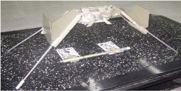
Fig. 8. The stereoscope and parallax ruler.
