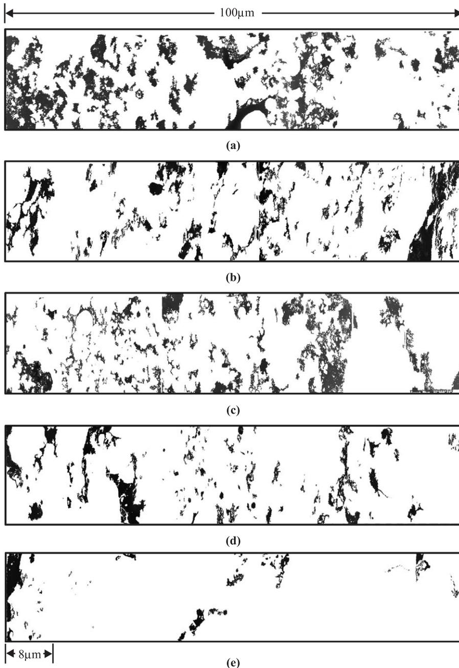
Fig. 11. The pore distribution of the transition zone of concrete curing with saturated lime water (W/B=0.54) at (a) 1 day (porosity=20.14%), (b) 7 days (porosity=16.55%), (c) 14 days (porosity=15.13%), (d) 28 days (porosity=9.93%) and (e) 56 days (porosity=3.51%).
