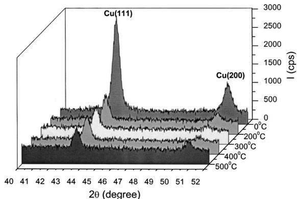
FIG. 2. X-ray diffraction patterns for as-deposited copper films and copper films annealed at the temperatures of 200, 300, 400, and 500 °C.
