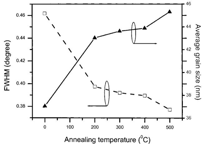
FIG. 3. Annealing temperature dependence of the FWHM of the (111) diffraction peaks of annealed copper films. Crystalline sizes for those annealed copper films were calculated as the Scherrer equation.
