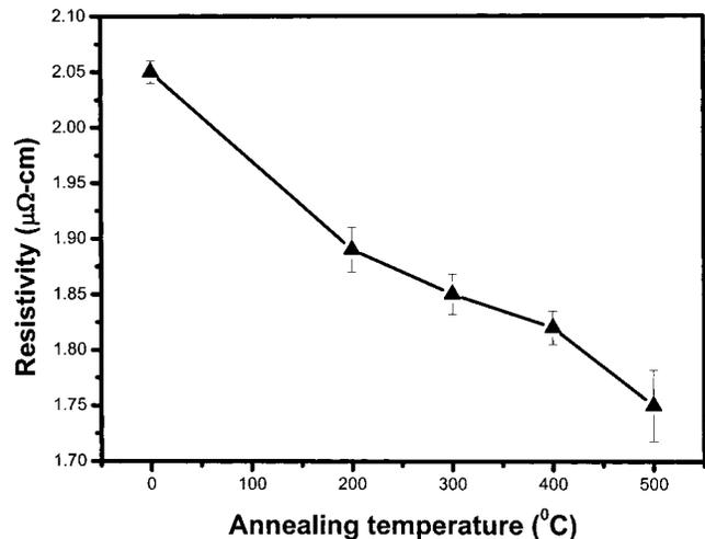
FIG. 6. Evolution of copper resistivity with the annealing temperatures.
