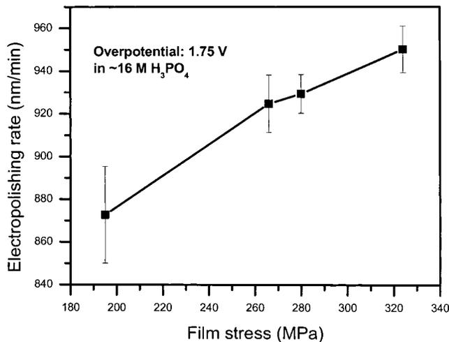
FIG. 5. Copper electropolishing rate for copper films with various stresses but with the same hardness and grain size.
