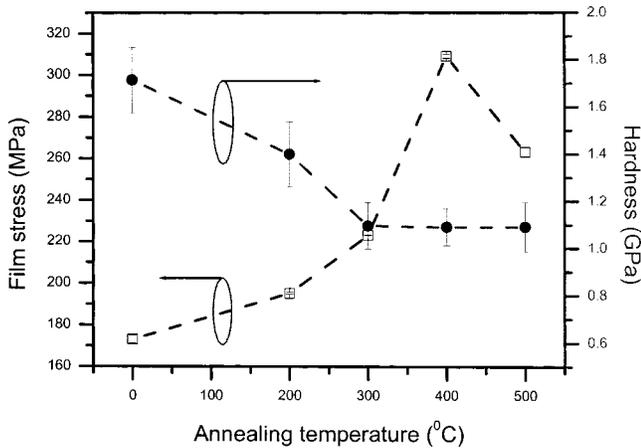
FIG. 1. Variation of film stress and hardness of copper films with the annealing temperature.
