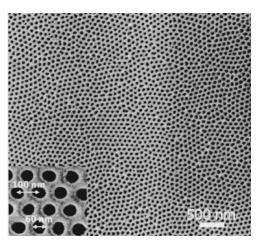
FIG. 2. Top-view SEM image of the nanoporous AAO film after pore widening in a H<sub>3</sub>PO<sub>4</sub> solution. The inset shows a close-up view of the hexagonal arrangement of the nanopores.
