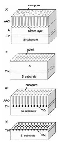
FIG. 1. Schematic diagram of the anodization process for fabrication of the titanium oxide nanodot arrays: (a) First anodic oxidation step, (b) prestructured Al film, (c) second anodization step and  $\mathrm{TiO}_x$  nanodot formation, and (d)  $\mathrm{TiO}_x$  nanodot arrays. The thickness of the electropolished Al film before anodic oxidation was about 4  $\mu$ m, and the sputtered TiN layer was 30 nm in thickness.
