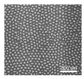
FIG. 4. Side-view SEM image of titanium oxide nanodot arrays after removing the nanoporous AAO template.
