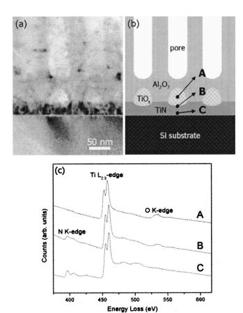
FIG. 3. (a) Cross-sectional TEM image of the bottom of AAO nanopore channels after the completion of the anodization, (b) diagrammatic illustration of the TEM image in (a), and (c) EELS spectra showing the Ti  $L_{2,3}$  edge, N K edge, and O K edge. The spectra correspond to three different positions as shown in (b): (A) At the center, (B) at the bottom, and (C) at the underside of the dome.
