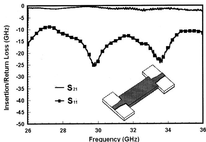
Fig. 5. Measured performance of the all-planar Ka-band transition.
