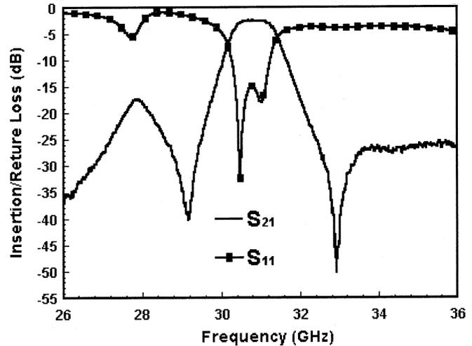
Fig. 3. Measured responses of Ka-band dual-mode filter with 1-GHz bandwidth.
