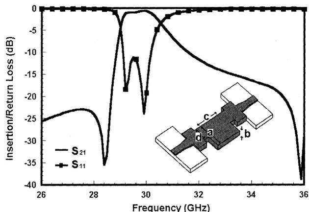
Fig. 1. Single-cavity dual-mode filter and its theoretical frequency responses. Each dual-mode cavity produces two transmission poles and one transmission zero. The parameters:  $a = 6.26$  mm,  $b = 0.508$  mm,  $c = 5.44$  mm,  $d = 2.5$  mm, and  $\epsilon_r = 3.38$ .
