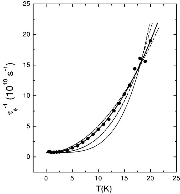
FIG. 3. Electron dephasing rate as a function of temperature for the PdAg17 thick film. The thick solid curve drawn through the data points is a least-squares fit to Eq. (1), using  $p$  as a free parameter. The dotted, dashed, and thin solid curves are least-squares fits to Eq. (1) with  $p$  fixed at 2, 3, and 4, respectively (see text).
