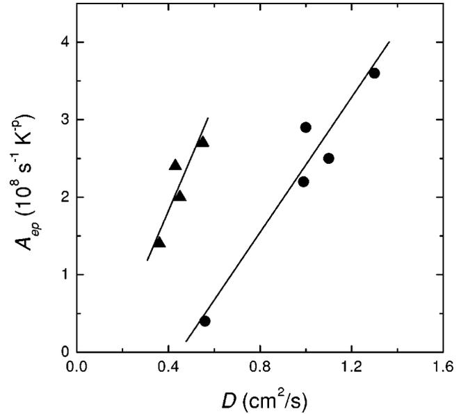
FIG. 4. The strength of  $e$ -ph coupling  $A_{ep}$  as a function of diffusion constant for dc- (triangles) and rf- (circles) sputtered PdAg thick films. The straight lines drawn through the data points are guides to the eye.
