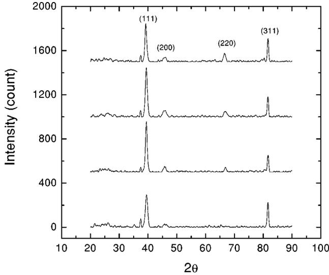
FIG. 1. X-ray diffraction patterns for two dc- (top two curves) and two rf- (bottom two curves) sputtered PdAg thick films. The sample resistivities  $\rho(300\text{ K})$  from top down are 189, 82, 79, and  $132\ \mu\Omega\text{ cm}$ . The diffraction intensity shows an arbitrary unit.
