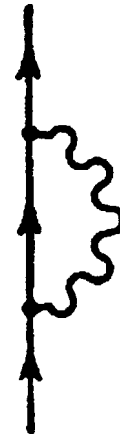
FIG. 1. O(e^2) correction to the electron propagator. Solid line: bare electron propagator, wavy line: photon propagator.
