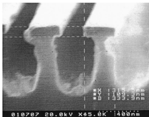
FIG. 9. SEM images of the etching profiles of a -C:F in O_2 plasmas (100 sccm) with bias power of 60 W (60 s).
