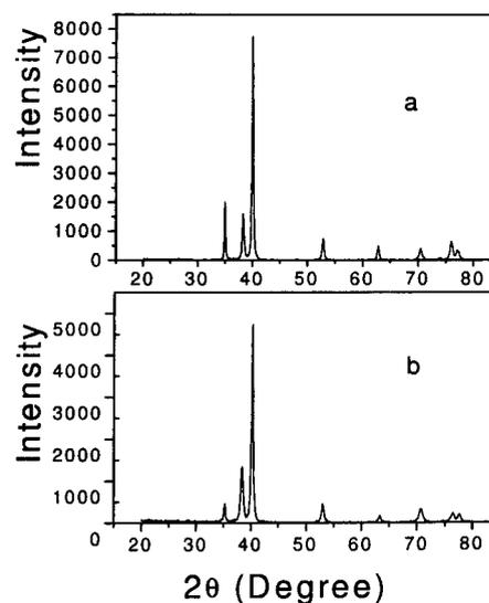
FIG.1 X-ray diffraction patterns of pure Ti (a) and Ti with 10 at. % Al (b). The patterns show that no preferential orientation exists in these two samples.
