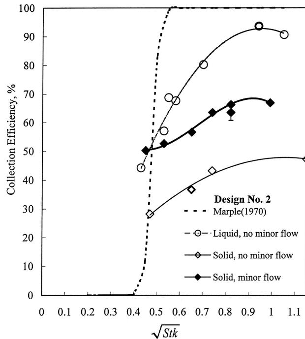
FIG. 7 Particle collection efficiency curve, design no. 2,  $S/W = 4.0$ .
