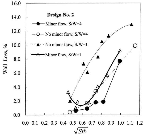
FIG. 8 Particle wall loss, design no. 2.
