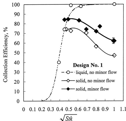
FIG. 3 Particle collection efficiency curve, design no. 1,  $S/W = 1.0$ .
