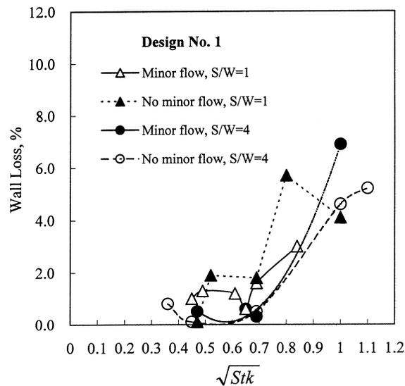
FIG. 5 Particle wall loss, design no. 1.
