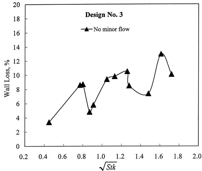
FIG. 10 Particle wall loss, design no. 3.
