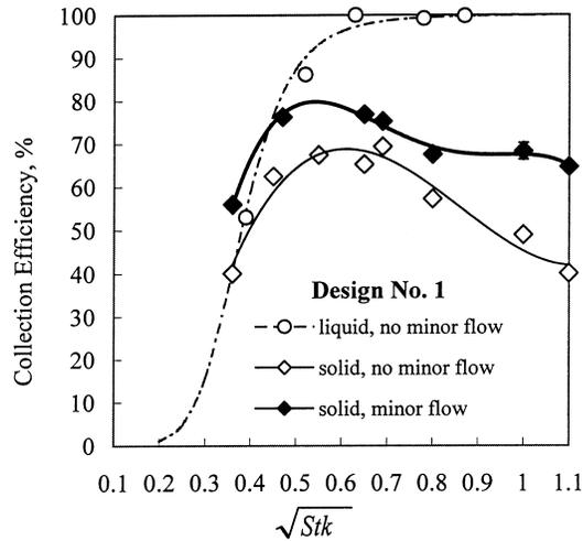
FIG. 4 Particle collection efficiency curve, design no. 1,  $S/W = 4.0$ .
