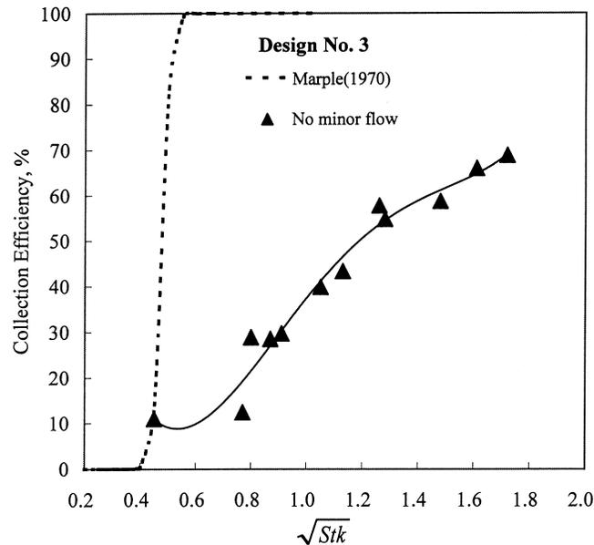
FIG. 9 Particle collection efficiency curve, design no. 3.
