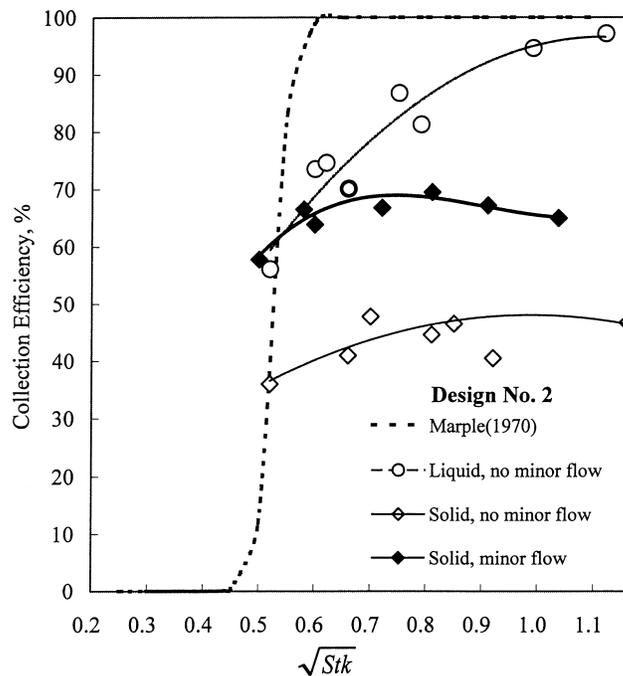
FIG. 6 Particle collection efficiency curve, design no. 2,  $S/W = 1.0$ .
