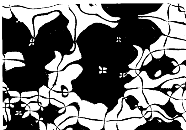
Figure 2. Optical polarizing micrograph displayed by 4M: nematic texture obtained after cooling from isotropic phase to -20 °C.
