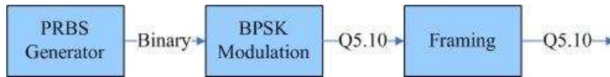
Figure 5.1: Fixed-point data formats used at different points in the ranging signal generator.
