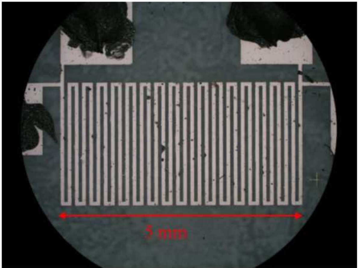
Figure 4.4: The picture of film which is fabricated by photolithography.
