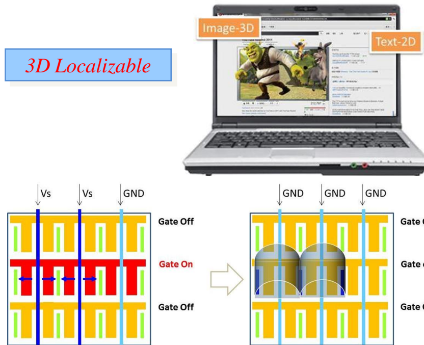
Fig. 5- 3 3D localized LC lens (a) gate on for side electrodes charging to middle electrodes (b) gate off for holding localized LC lens
