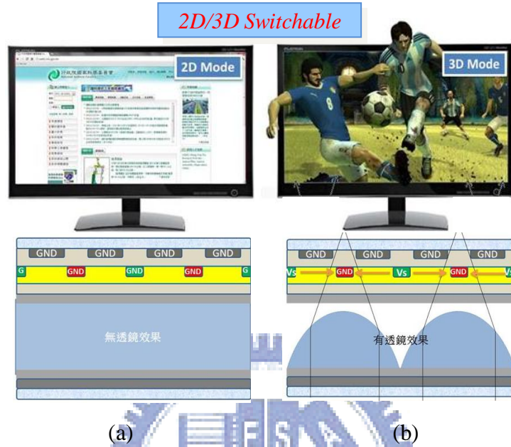
Fig. 5- 1 2D/3D switchable LC lens (a) lens off (b) lens on
