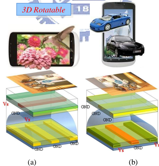
Fig. 5- 2 3D rotatable LC lens (a) driving top electrodes for horizontal 3D images (b) driving bottom electrodes for vertical 3D images
