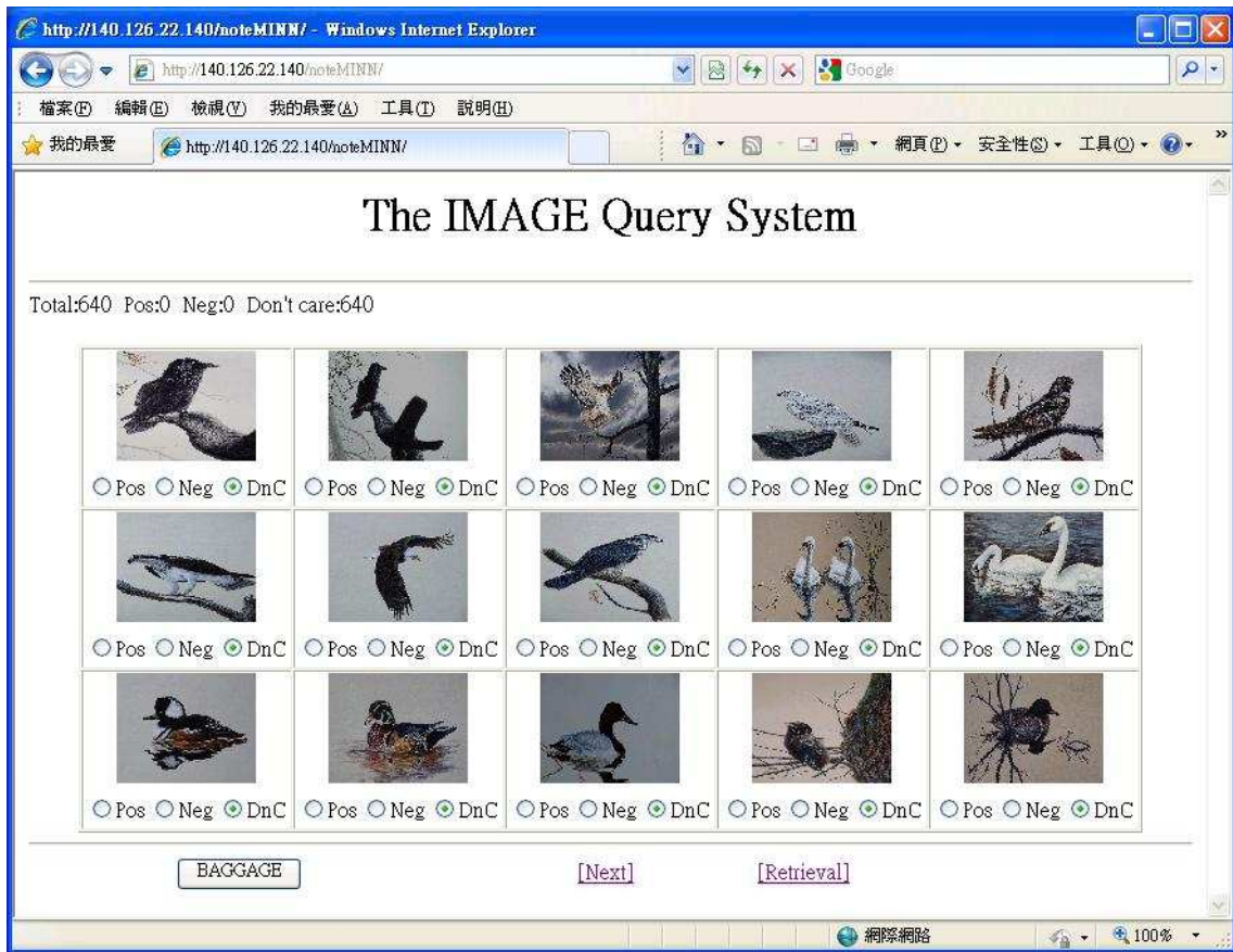
Figure 5.2: The prototype system of the IMAGE Query System. When a user enters the system, one can select a class on interested of images with Pos or Neg radio button.
