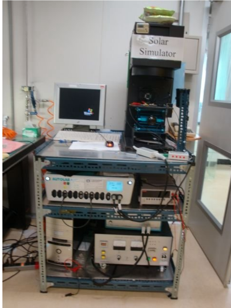
Figure 3.3 The appearance of Yamashita Denso solar simulator (YSS-100A).
