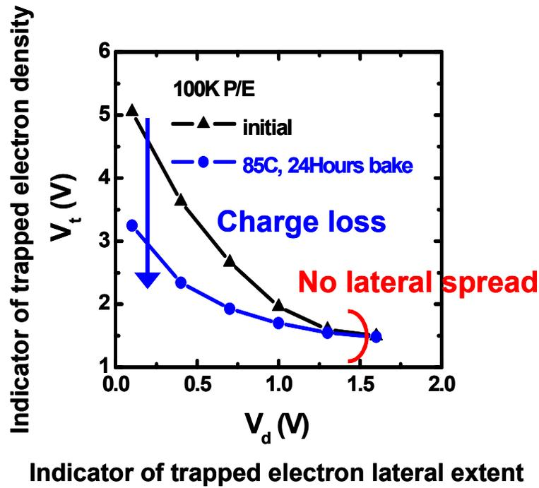
Fig.2.5 The measured  $V_t$  versus  $V_d$  characteristics of a 100K P/E cycled cell before and after 24 hours, 85C storage. The cell is at program state.
