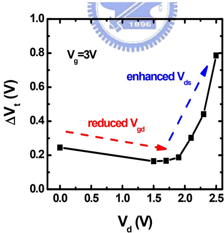
Fig.5.8 Read disturb induced  $V_t$  shift versus applied drain bias of a 10K P/E cycled cell. The disturb time is  $10^4$  sec.  $V_g/V_s=3V/0V$  and  $L_g=0.5\mu m$ .
