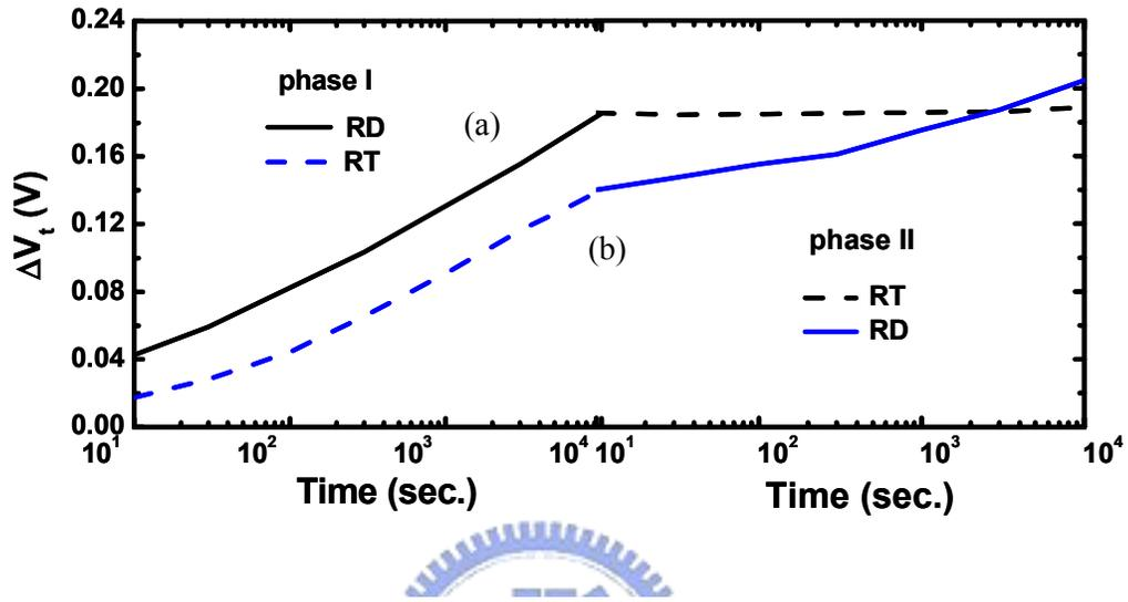
Fig.5.2 Two-phase measurement of the  $V_t$  shift temporal evolution of a 10K P/E cycled cell. In curve (a), the cell is at RT mode in the first  $10^4$  sec. and is at RD mode in the following  $10^4$  sec. The sequence is reversed in curve (b). Bias conditions of RT and RD are  $V_g/V_d/V_s=0V/0V/0V$  and  $V_g/V_d/V_s=3V/1.6V/0V$ , respectively.  $L_g=0.5\mu m$ .
