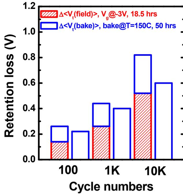
Fig.2.19 Overall retention loss of various cycled sectors by 150C, 50 hours bake ( $\Delta\langle V_t(\text{bake}) \rangle$ ) with and without a preceding field acceleration of  $V_g = -3V$ , 18.5 hours ( $\Delta\langle V_t(\text{field}) \rangle$ ).
