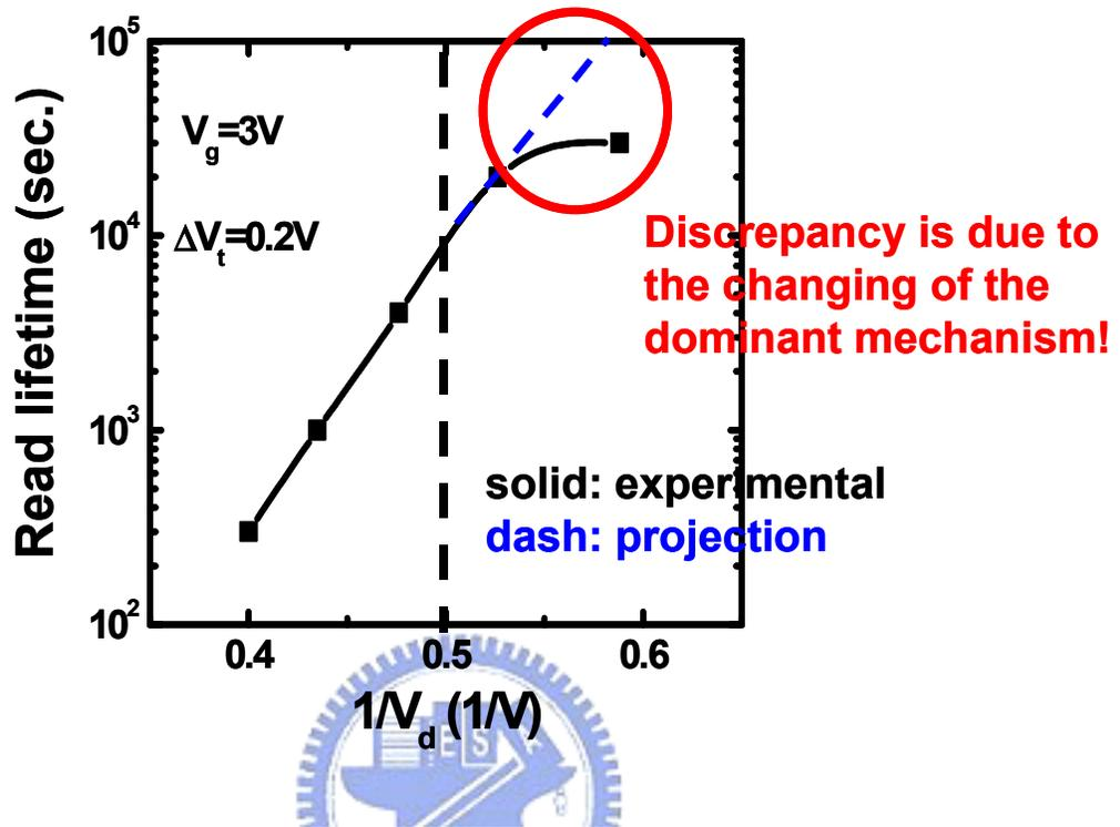
Fig.5.9 Read lifetime projection by  $V_d$ -accelerating approach. Lifetime is defined as the disturb time resulting in a  $V_t$  shift of 0.2V.  $V_g/V_s=3V/0V$  and  $L_g=0.5\mu m$ . As shown in the figure, lifetime is overestimated in the low- $V_d$  regime where gate-enhanced disturb dominates.
