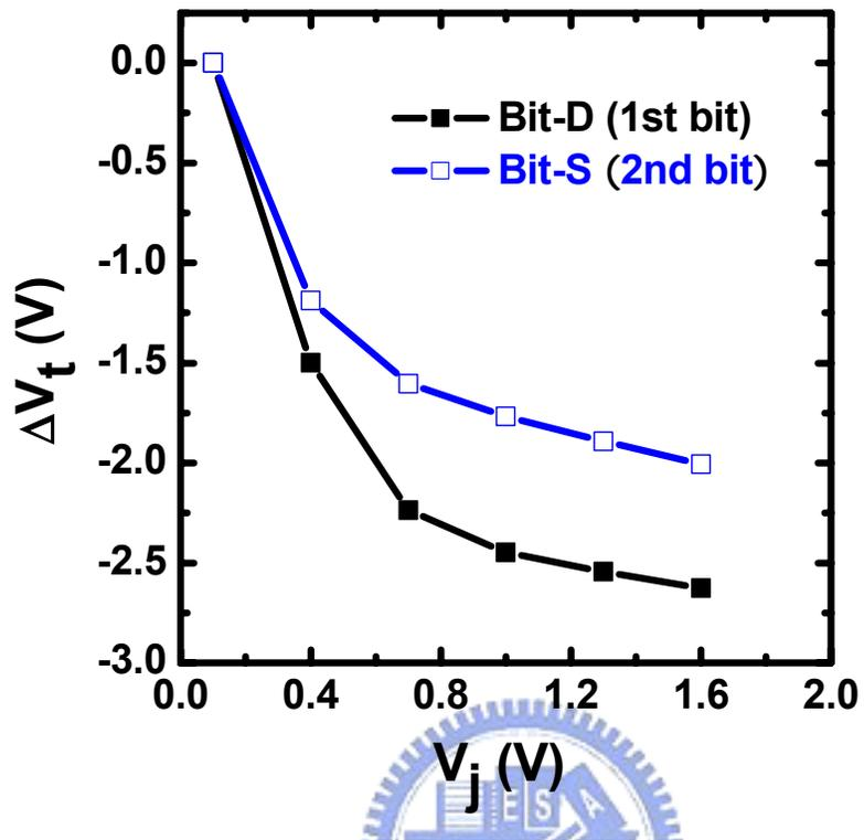
Fig. 6.5  $\Delta V_t$ - $V_j$  measurement of the Bit-D and the Bit-S of an NBit cell.  $V_j$  is equal to  $V_d$  for Bit-D, and is equal to  $V_s$  for Bit-S. This result is at the 50<sup>th</sup> cycle.
