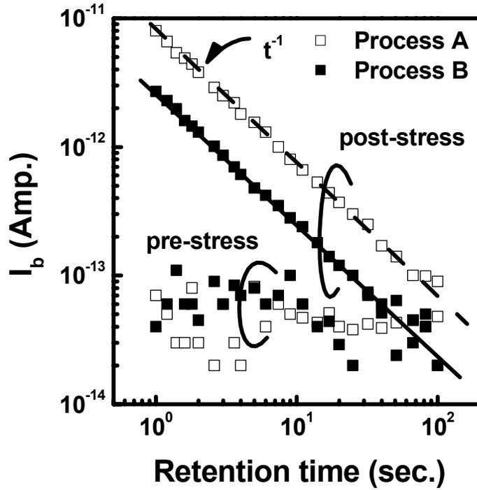
Fig.3.9 Pre-stress and post-stress substrate currents in two large area devices ( $500\mu\text{m} \times 500\mu\text{m}$ ). The FN stress condition is  $V_g = -18\text{V}$  for 3000s. Substrate current was measured at  $V_g = V_{fb}$ .
