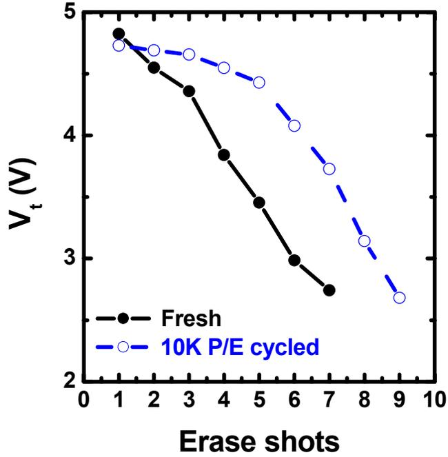
Fig.4.4 The required erase time versus cycle numbers of an emulating single cell.
