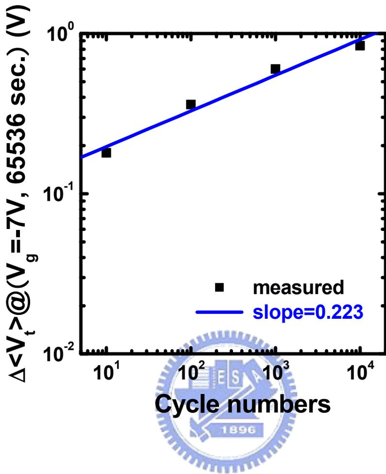
Fig.2.17  $\Delta\langle V_t \rangle$  by field acceleration versus cycle numbers in a product.
