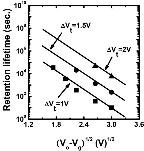
Fig.2.12 The charge retention lifetime versus  $(V_0 - V_g)^{1/2}$ . Retention lifetime is defined as the storage time sustained for  $\Delta V_t = 1V, 1.5V,$  and  $2V,$  respectively.
