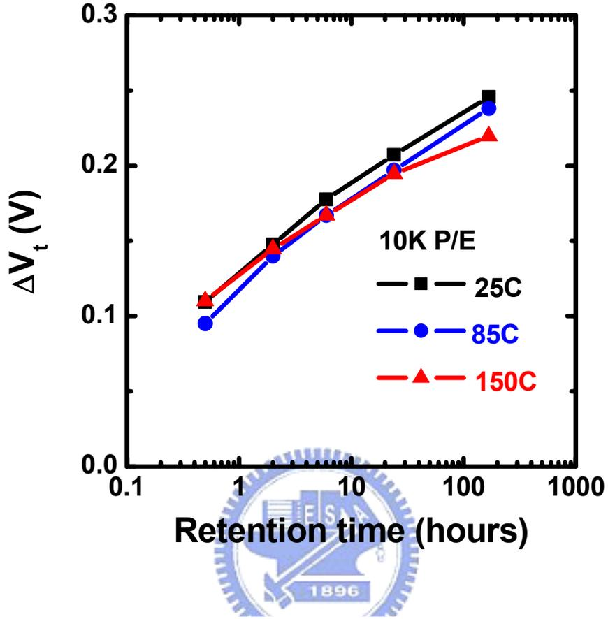
Fig.3.2 The  $V_t$  shift versus the retention time of 10K P/E cycles cells in erase state. The bake temperatures are 25C, 85C, and 150C.
