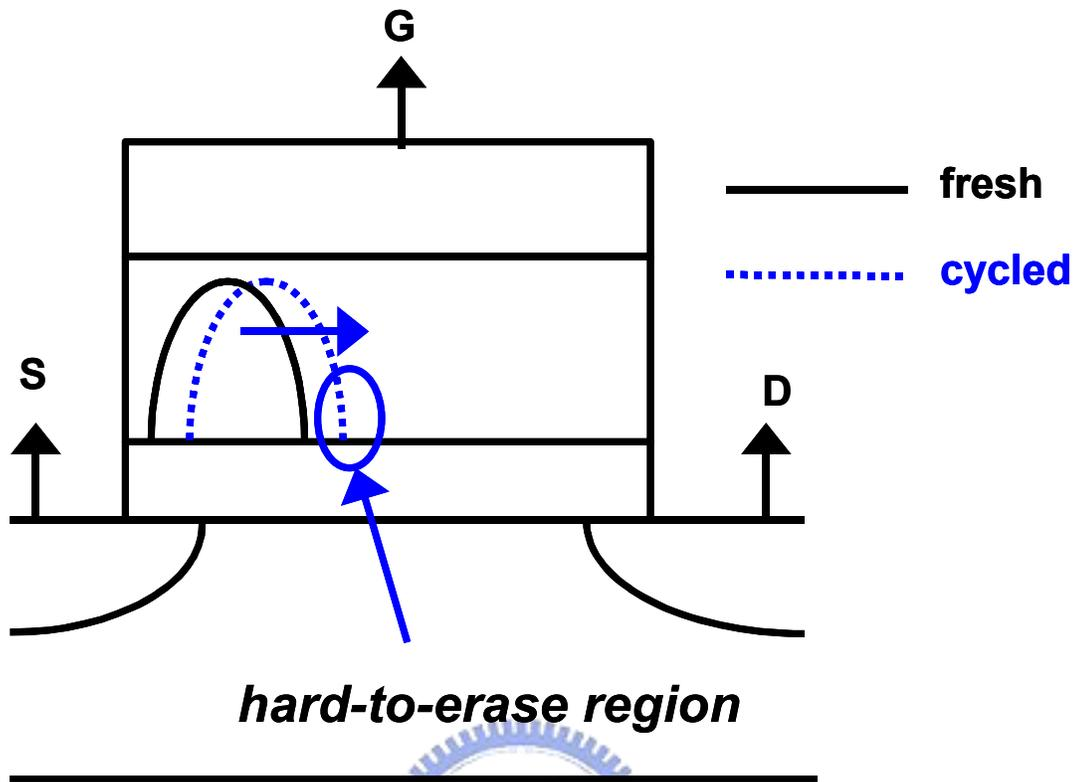
Fig.6.10 Schematic representation of the injected electron distribution after programming of a fresh and a 50 P/E cycled NBit cells.
