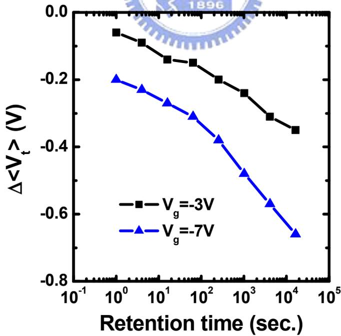
Fig.2.16  $\Delta\langle V_t \rangle$  evolution with  $V_g$ -accelerating time of a 10K cycled sector.  $V_g = -3V$  and  $-7V$ .
