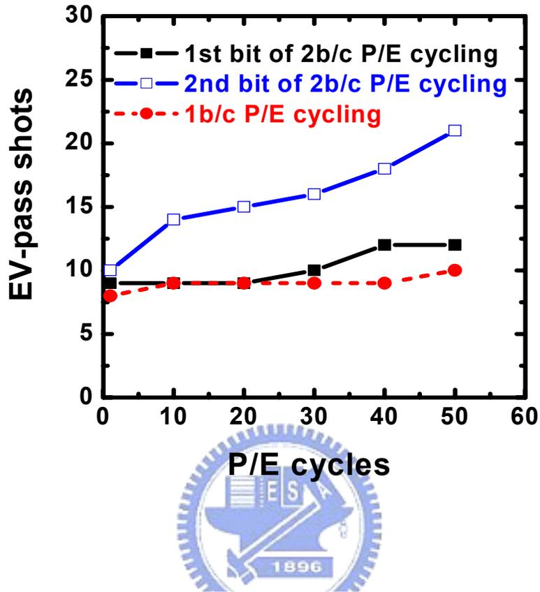
Fig.6.1 EV-pass shot v.s. cycles of a 2Mb test chip. Here, the EV-pass shots mean the accumulated erase shots necessary for all the 1<sup>st</sup> or the 2<sup>nd</sup> bits of the chip to pass erase-verify (EV).
