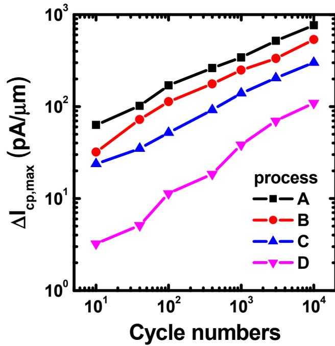
Fig.2.25 Normalized  $\Delta I_{cp,max}$  versus cycle numbers of NBit cells fabricated by various process conditions.
