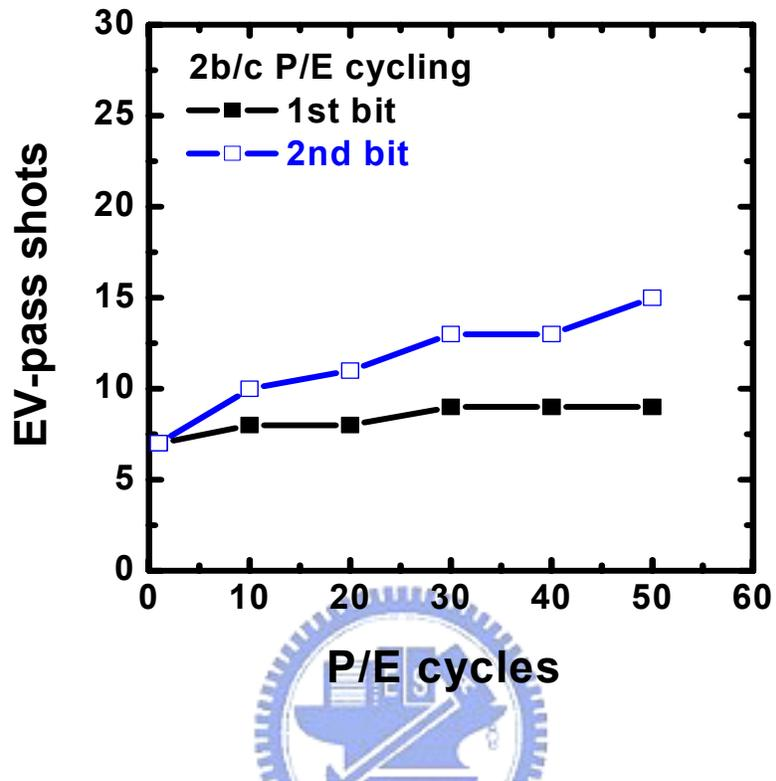
Fig.6.4 EV-pass shots v.s. P/E cycles of an NBit cell.
