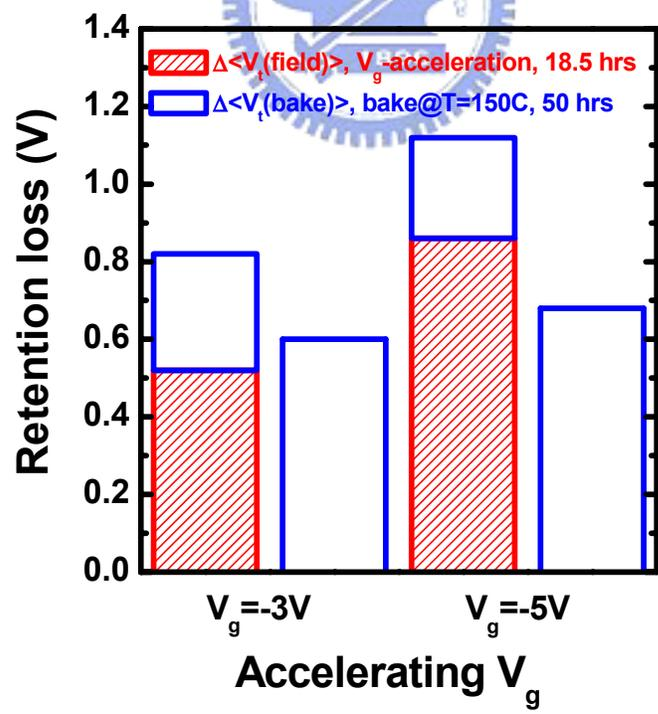
Fig.2.20 Overall retention loss of 10K cycled sectors by 150C, 50 hours bake ( $\Delta\langle V_T(\text{bake}) \rangle$ ) with and without a preceding 18.5 hours field acceleration of  $V_g = -3V$  and  $-5V$  ( $\Delta\langle V_t(\text{field}) \rangle$ ).
