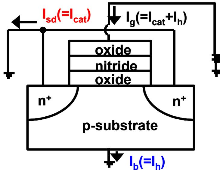
Fig.3.7 Illustration of a charge separation technique.  $I_{sd}$  is an electron leakage current and  $I_b$  is a hole leakage current.
