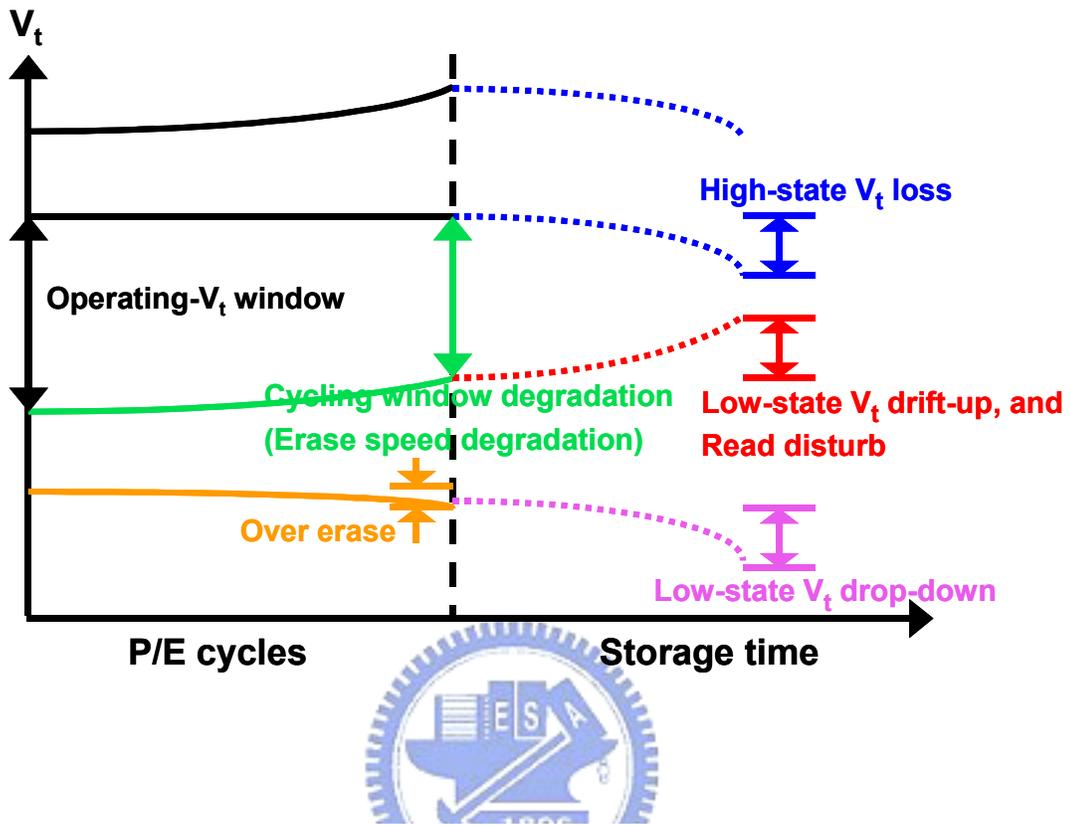
Fig.1.10 Representation of the reliability issues we have observed in an NBit cell.
