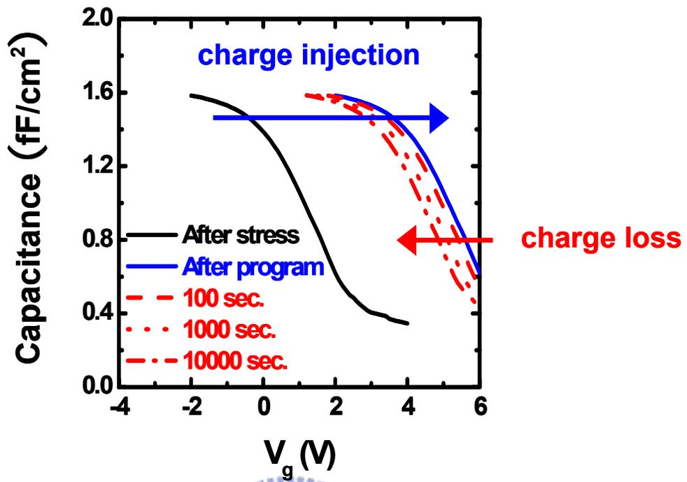
Fig.2.8 The CV temporal evolution of an ONO capacitor.
