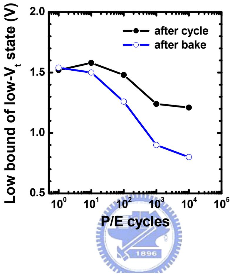
Fig.4.1 The low bound of erase-state  $V_t$  distribution versus cycle numbers before and after baking at 150C for 168 hours.
