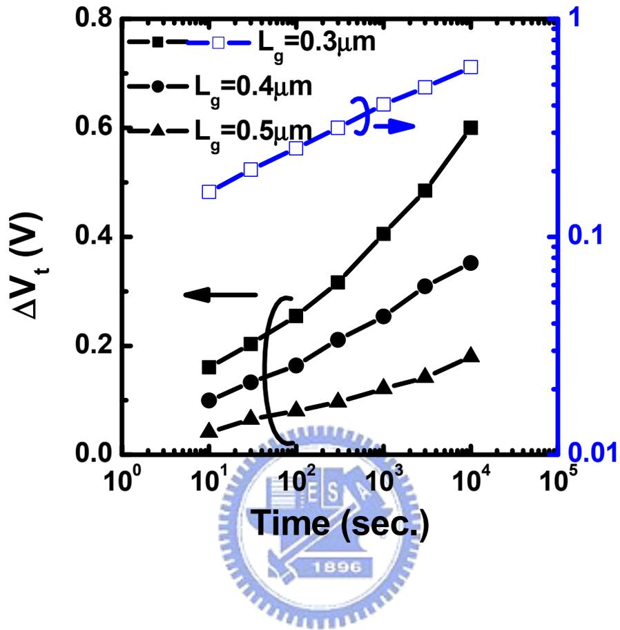
Fig.5.10  $V_t$  shift versus disturb time of 1K P/E cycled cells with different channel lengths.  $V_g/V_d/V_s=3V/1.6V/0V$ .
