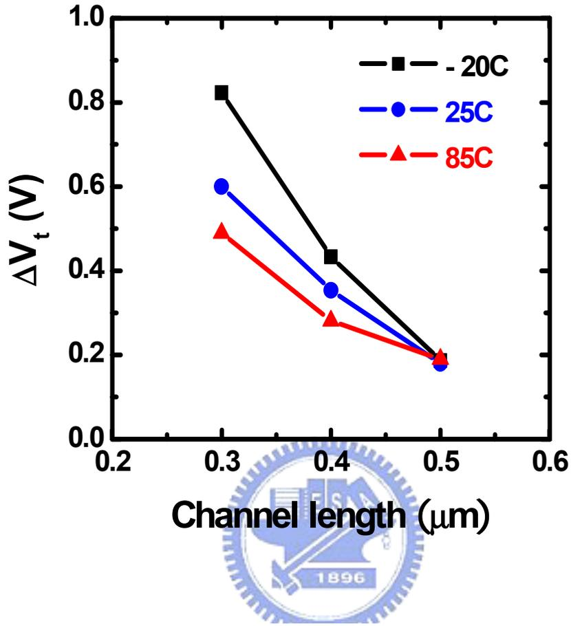
Fig.5.11 Temperature effect on read disturb of 1K P/E cycled cells. Devices with gate lengths of 0.5 $\mu\text{m}$ , 0.4 $\mu\text{m}$  and 0.3 $\mu\text{m}$  are characterized. The applied gate and drain biases are 3V and 1.6V, respectively, and the disturb time is 10<sup>4</sup> sec..
