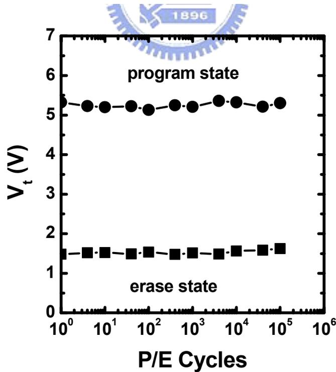
Fig.1.8 Endurance characteristics of an NBit cell.
