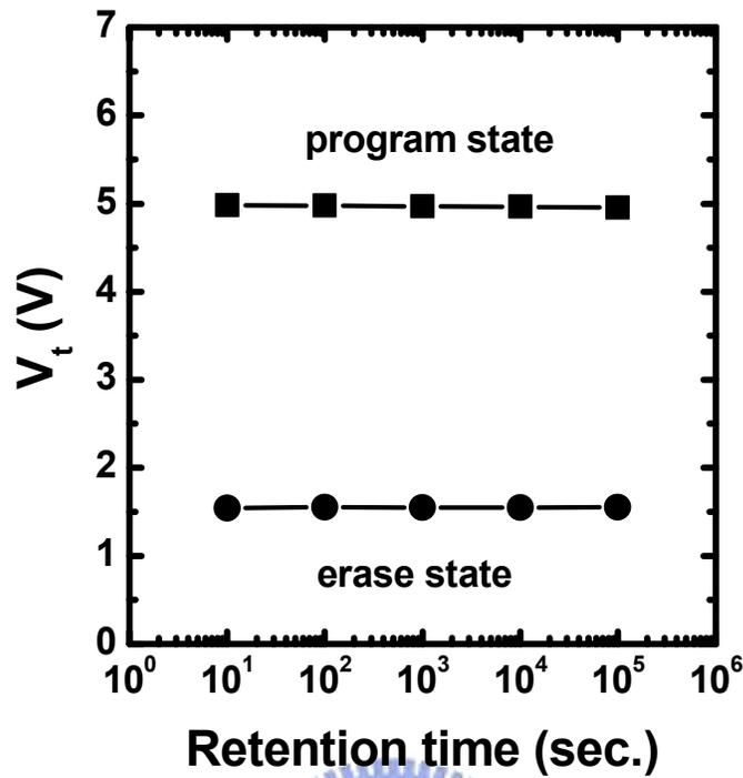
Fig.1.7  $V_t$  versus retention time of a fresh NBit cell. The bake temperature is 150C.
