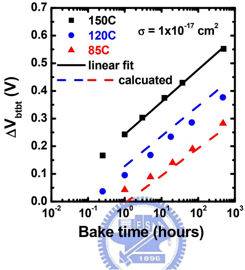
Fig.4.10  $\Delta V_{bibt}$  versus bake time at various temperatures. All curves follow a straight line on a semi-log scale. The lines represent the calculated results.
