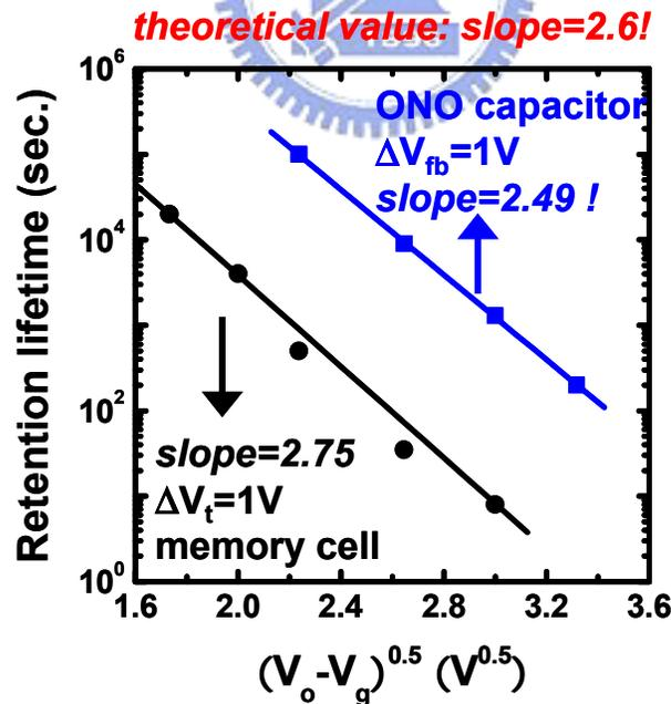
Fig.2.13 The retention lifetime versus  $(V_0 - V_g)^{1/2}$ .  $V_0$  is  $2V$  and  $5V$  for the cell and the capacitor, respectively. The retention lifetime is defined as the storage time sustained for a  $1V$  shift of the  $V_{fb}$  of the capacitor or a  $1V$  shift of the  $V_t$  of the memory cell.
