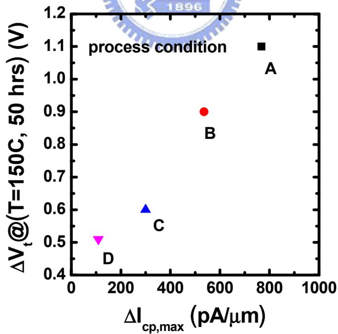
Fig.2.26  $\Delta V_t$  by high-temperature bake versus  $\Delta I_{cp,max}$  of 10K cycled cells of various processes.
