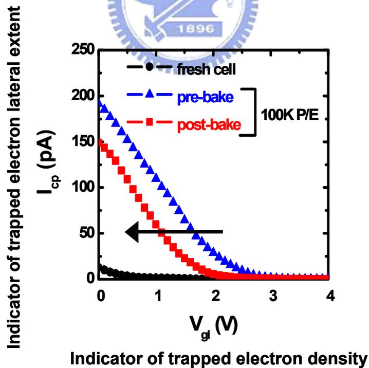
Fig.2.6 The measured charge-pumping current ( $I_{cp}$ ) versus the low level of gate pulse ( $V_{gl}$ ) in the CP measurement. The 100K cycled cell is at program state. The bake time is 24 hours and the bake temperature is 85C.
