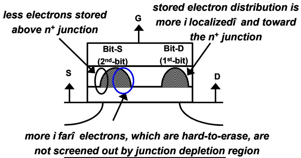
Fig.6.2 Schematic representation of an NBit cell structure and localized charges storage. The charge distributions are depicted for the case in which Bit-D is the 1<sup>st</sup> bit and Bit-S is the 2<sup>nd</sup> bit.
