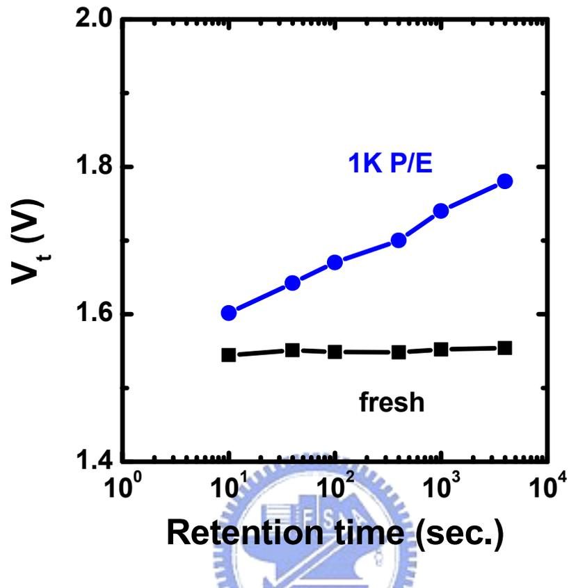
Fig.3.1 Erase-state  $V_t$  drift versus retention time of a fresh and a 1K P/E cycled NBit cells.
