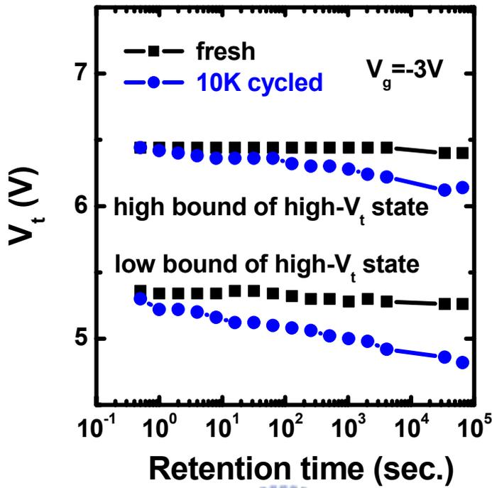
Fig.2.15  $V_t$  evolution with  $V_g$ -accelerating time of a fresh and a 10K cycled sectors.  $V_g = -3V$ .
