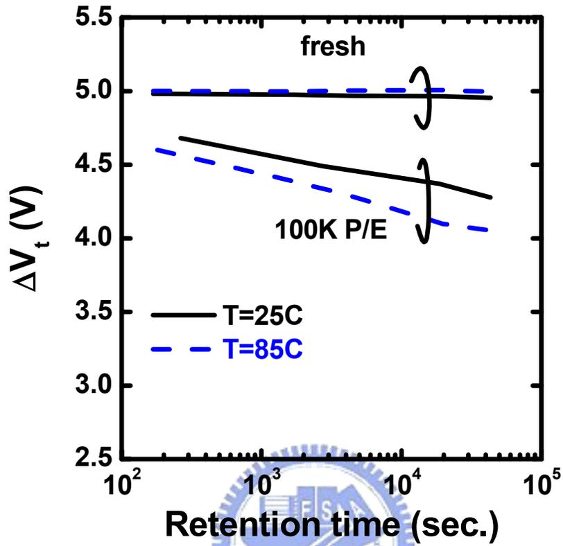
Fig.2.2 Program-state charge loss versus retention time in a fresh and a 100K P/E cycled NBit cells. T=25C and 85C.
