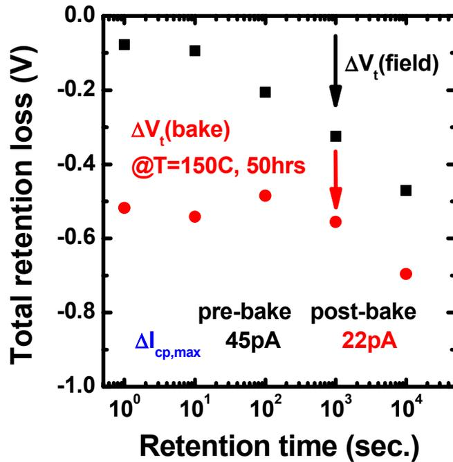
Fig.2.21 The retention loss of a 10K cycled cell, which is firstly accelerated by  $V_g=-3\text{V}$  for various time and then baked at  $T=150\text{C}$  for 50 hours, is recorded. The variation of  $\Delta I_{\text{cp,max}}$  is also denoted.
