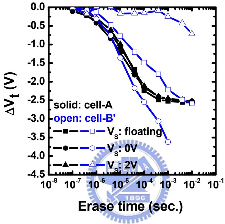
Fig.6.12 Erase speed comparison among various source junction biases during erasing the Bit-D of cell-A and cell-Bi.  $V_g/V_d=-6V/5V$ .
