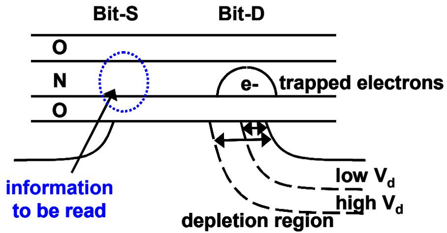
Fig.1.2 Concept of reverse read is depicted by the drain depletion region in which the effect of injected charges is screened out.
