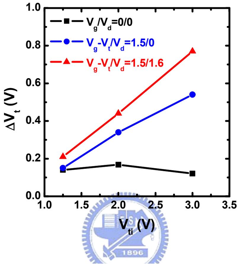
Fig.5.12 Initial threshold voltage versus room-temperature drift, gate disturb and read disturb. The cells undergo 10K P/E cycles. The bias conditions for GD, and RD are  $V_g-V_{ti}/V_d/V_s=1.5V/0V/0V$  and  $1.5V/1.6V/0V$ , respectively, and  $V_g=V_d=V_s=0V$  for RT. The disturb time is  $10^4$  sec. and  $L_g=0.5\mu m$ .
