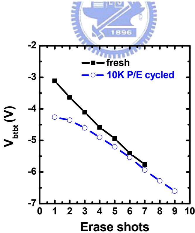
Fig.4.5 The extracted  $V_{btbt}$  versus cycle numbers corresponding to Fig.4.4.
