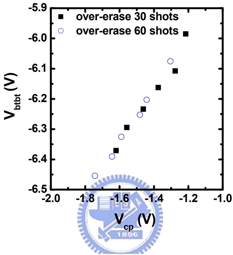
Fig.4.8  $V_{btbt}$  is plotted against  $V_{cp}$ . A positive correlation is found between them.
