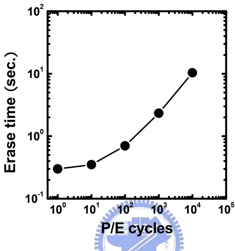
Fig.4.3 The required erase time versus cycle numbers corresponding to Fig.4.1.
