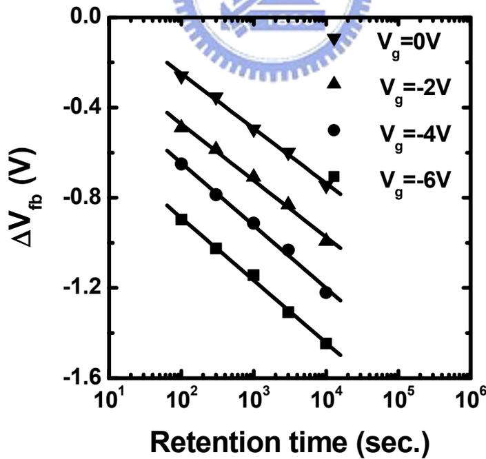
Fig.2.9 Evolution of the flatband voltage shift with the retention time in an ONO capacitor. The gate biases in measurement are 0, -2V, -4V, and -6V.
