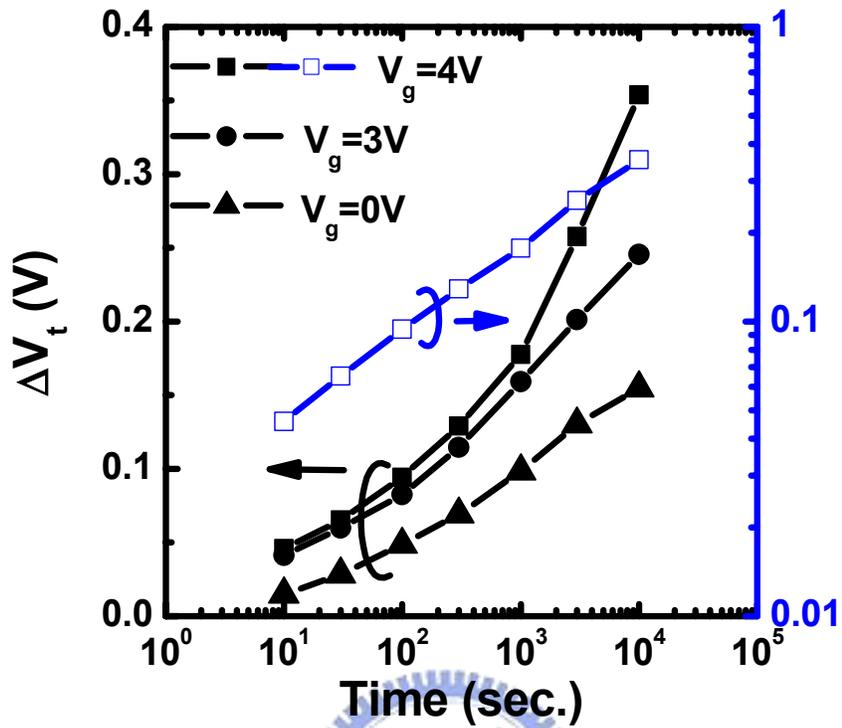
Fig.5.4  $V_t$  shift versus applied gate bias of a 10K P/E cycled cell. The drain and the source are grounded, and the disturb time is  $10^4$  sec.  $L_g=0.5\mu\text{m}$ .
