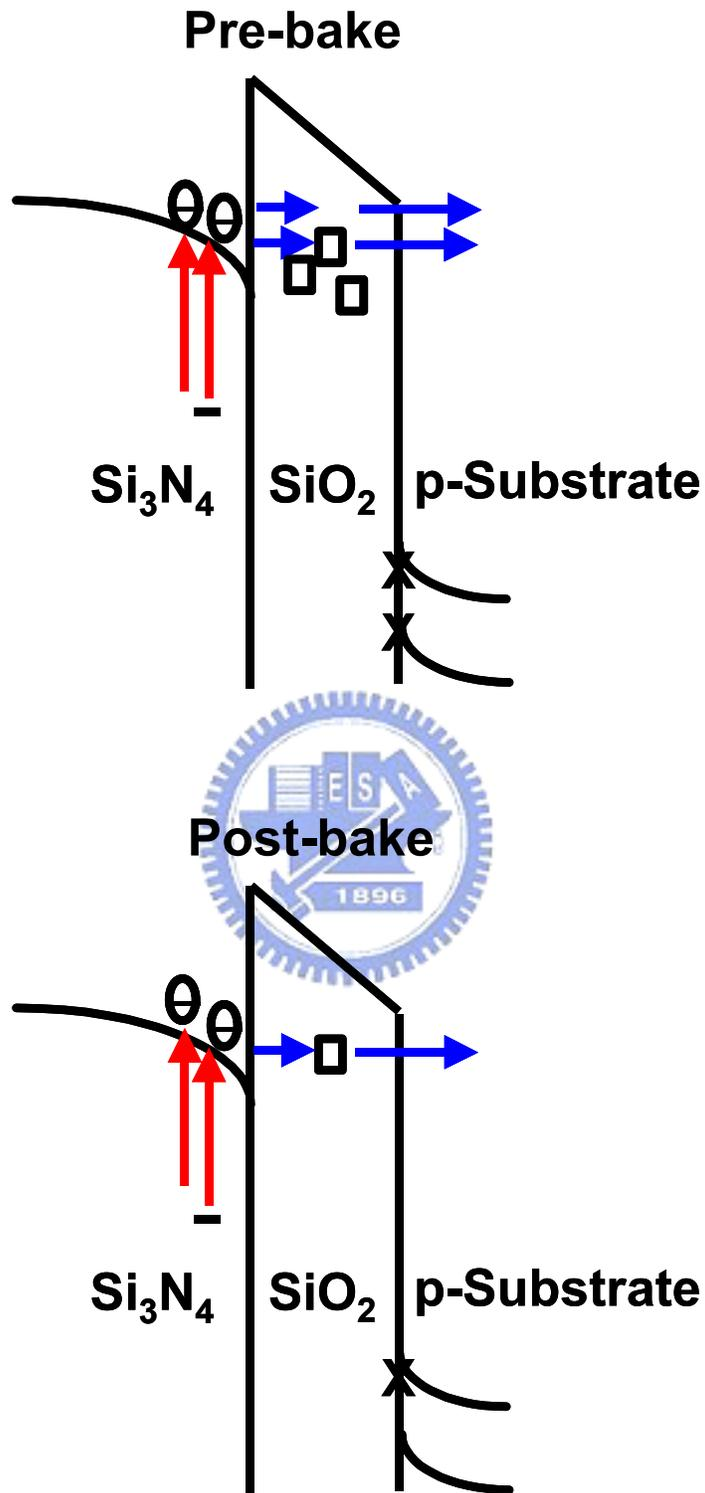
Fig.2.23 Roles of oxide trap and interface state in the retention loss of an NBit cell.
