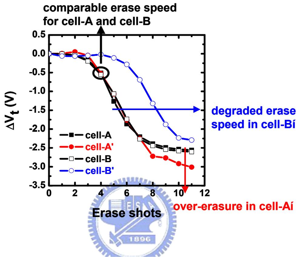
Fig.6.11 Erase characteristics of cells of various  $L_g$  and  $V_{ti}$  (Table 6.1).  $\Delta V_t$  representation the  $V_t$  shift from its programmed-state is  $V_t$  after each erase shot.
