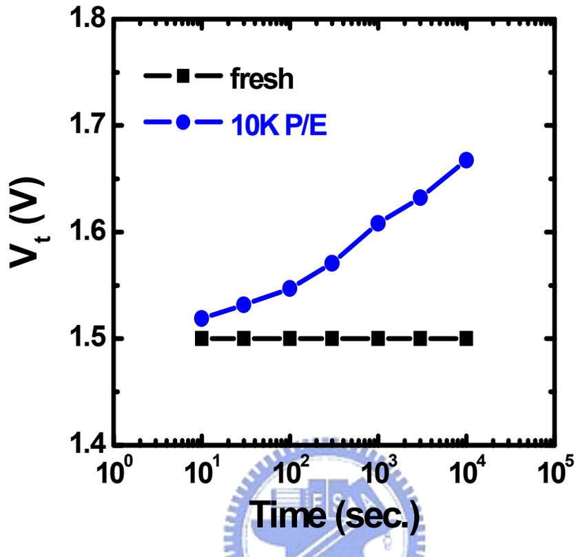
Fig.5.1 Read disturb characteristics of a fresh cell and a 10K P/E cycled cells.  $L_g=0.5\mu\text{m}$  and  $V_g/V_d/V_s=2.5\text{V}/1.6\text{V}/0\text{V}$ .
