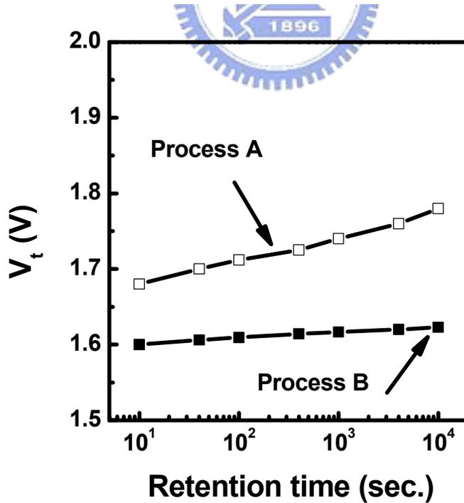
Fig.3.10 Room-temperature  $V_t$  drift versus time in two 10K P/E cycled cells fabricated with different ONO processes. The cell size is  $L_g = 0.5\mu\text{m}$  and  $W_g = 0.35\mu\text{m}$ .
