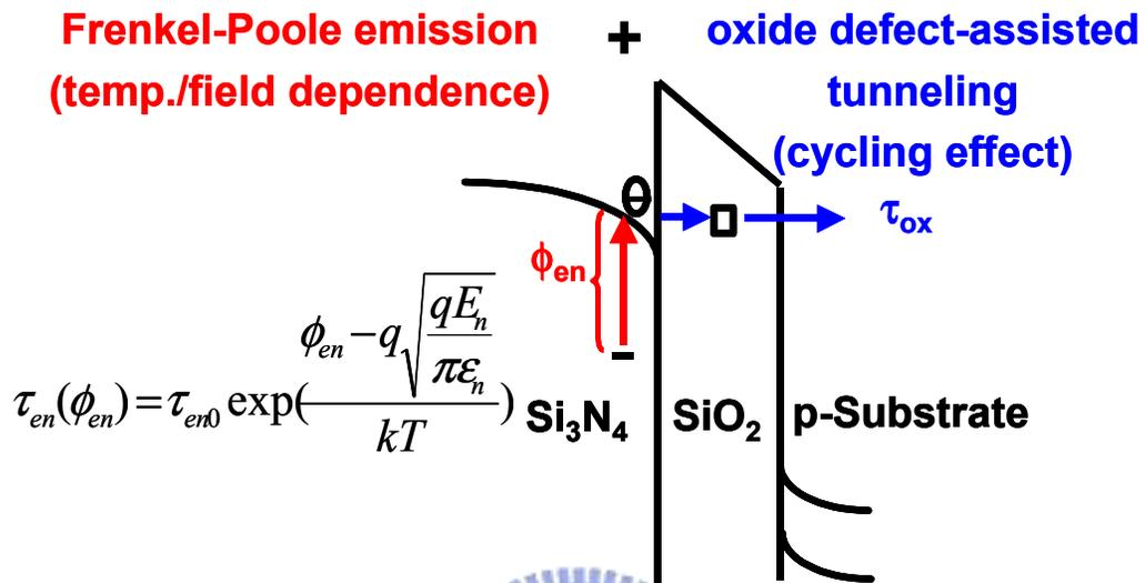
Fig.2.10 Illustration of nitride trapped charges escape via Frenkel-Poole emission and subsequent oxide defect-assisted tunneling.
