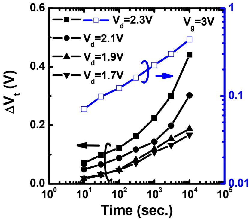
Fig.5.7  $V_t$  shift versus disturb time of a 10K P/E cycled cell at various drain biases.  $V_g/V_s=3V/0V$  and  $L_g=0.5\mu m$ .
