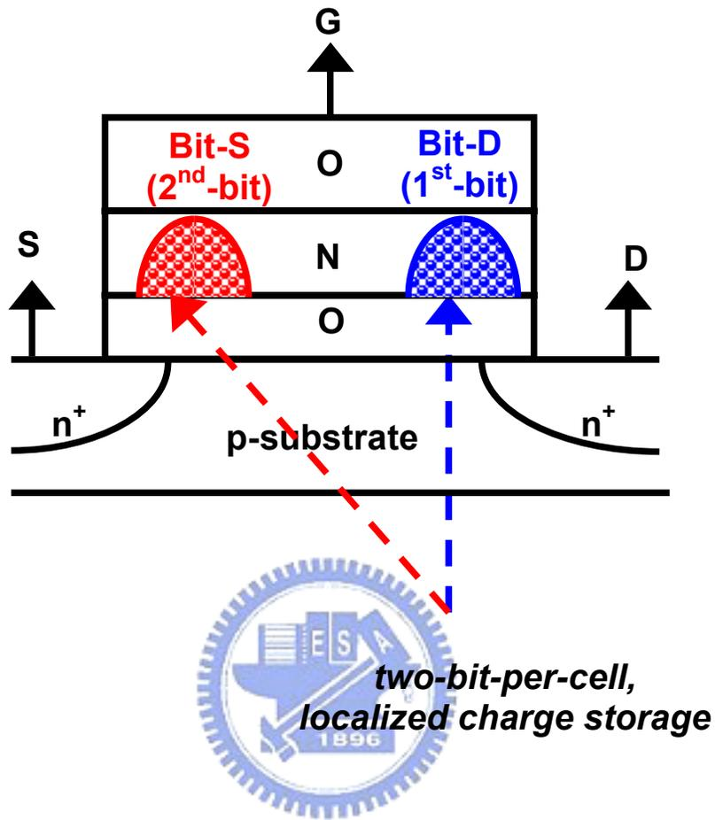
Fig.1.1 Schematic representation of an NBit cell.
