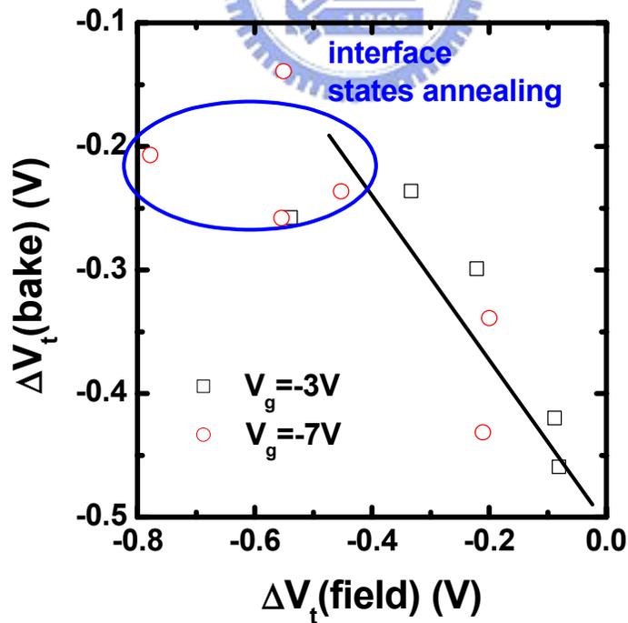
Fig.2.22 (Following)  $\Delta V_t(\text{bake})$  versus (preceding)  $\Delta V_t(\text{field})$  of 10K cycled cells. Bake is at  $150\text{C}$ , 50 hours, and field acceleration is done by  $V_g=-3\text{V}$  and  $\approx 7\text{V}$  with various retention time.
