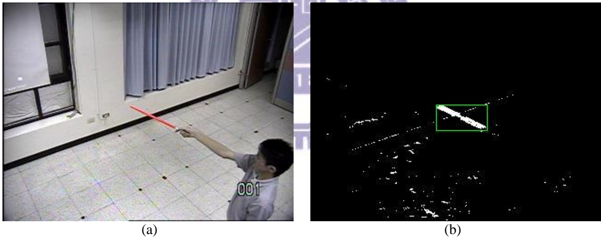
Fig. D.1. (a) An input image. (b) The detected pointer and its bounding box.
