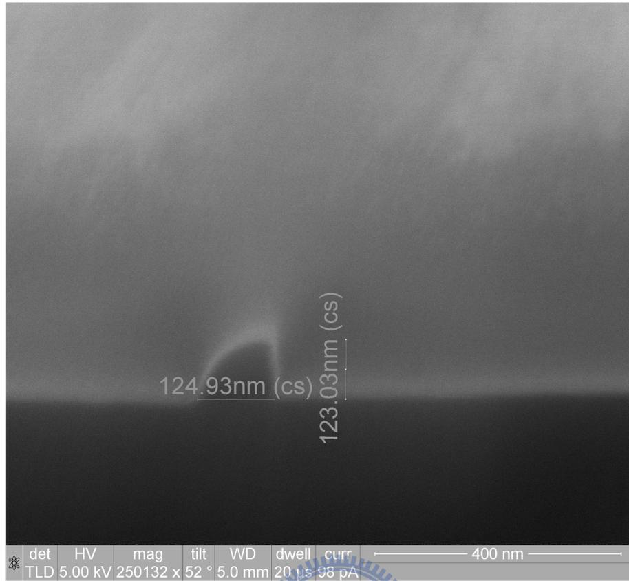
Fig. 4.1 Cross sectional view of a Green Transistor
