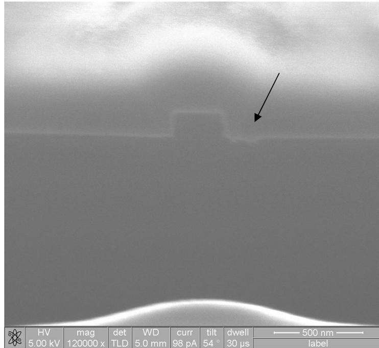
Fig. 3.16 Cross-sectional view of a 0.3  $\mu\text{m}$  MOSFET showing an etch-induced recess in the drain region.
